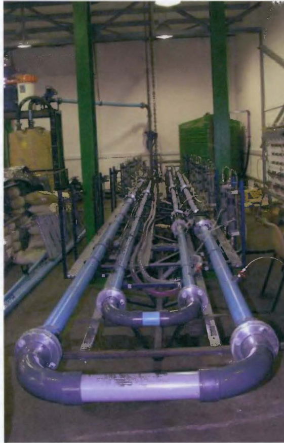
Figure 2.5: FPRC pipe test loop
