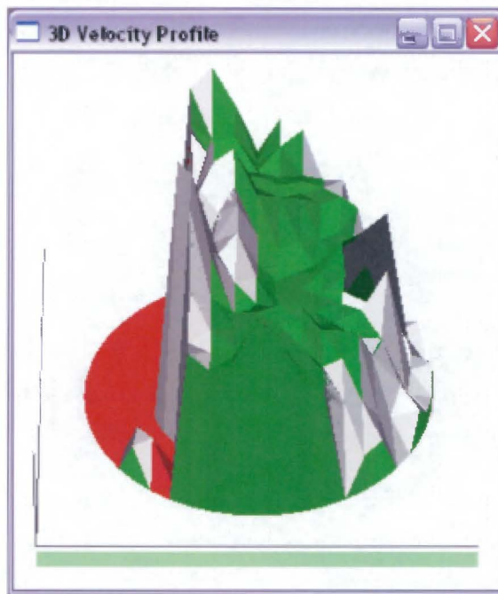
Figure 6.13: Interpolating across pixels with low correlation coefficients
