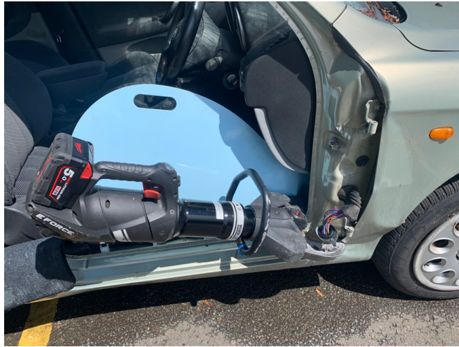
FIGURE 9.2: PHOTOGRAPH DEMONSTRATING RELIEF CUT POSITION
