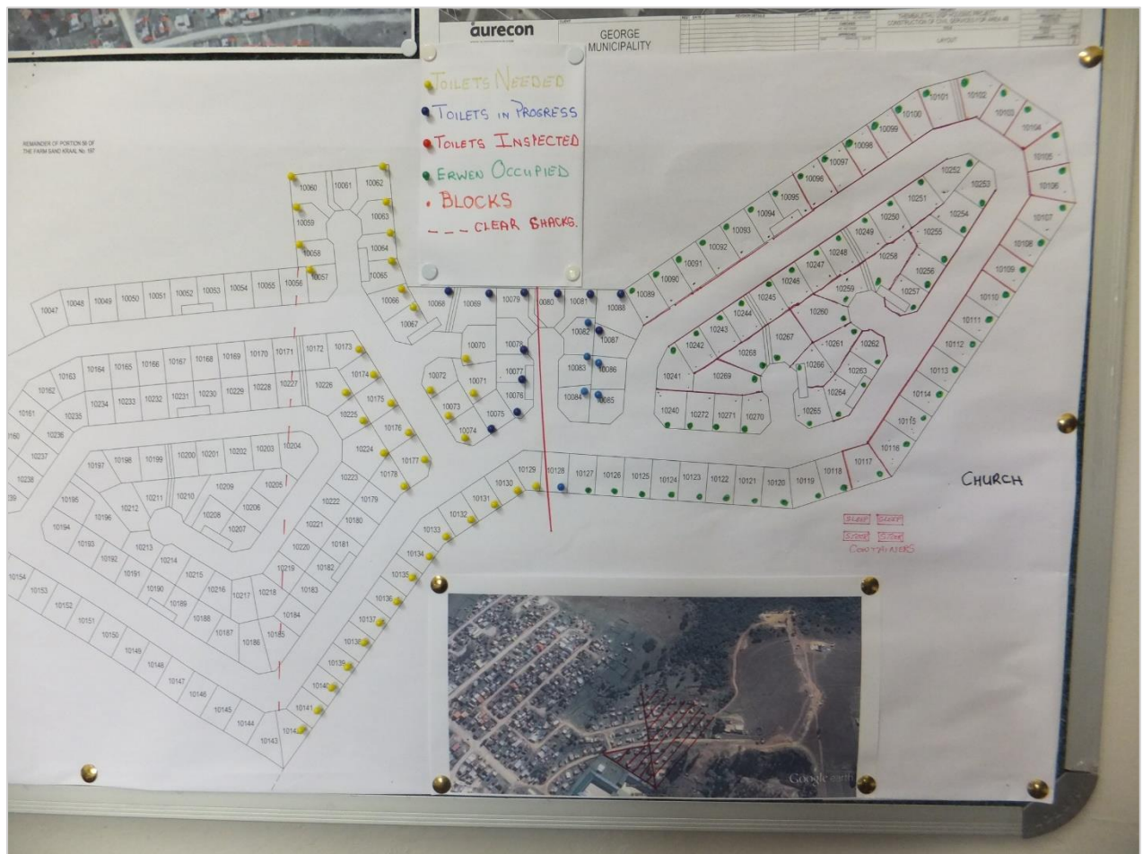
Image R: This Map indicates the progress of services during the construction (service sites) phase of Area 4 B on or by a specific date. This helps the team navigate, and, more importantly, visualise what has been already done and what is still needing to be done (Aurecon, 3/20/2014)
