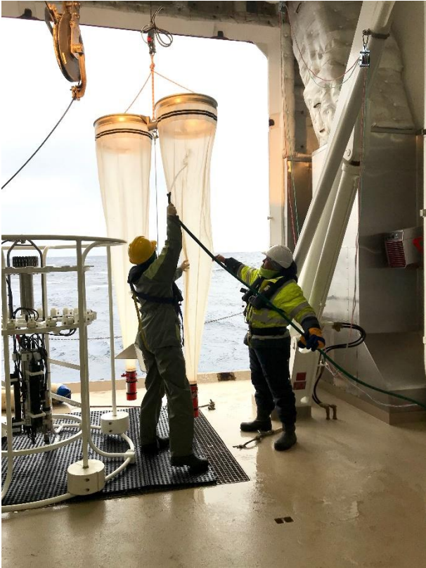
Figure 1.15 On board of the MV S.A. Agulhas II : (Centre) Plankton sample collection using a Bongo net requires rigorous net washing for plankton concentration in the Bongo net's cod-end. (Left) The Conductivity Temperature Depth (CTD) profiling instrument, crucial for determining the physical properties of seawater, is affixed to the rosette frame, which can also hold Niskin bottles used for water sampling (photo taken by Sina Wallschuss).
