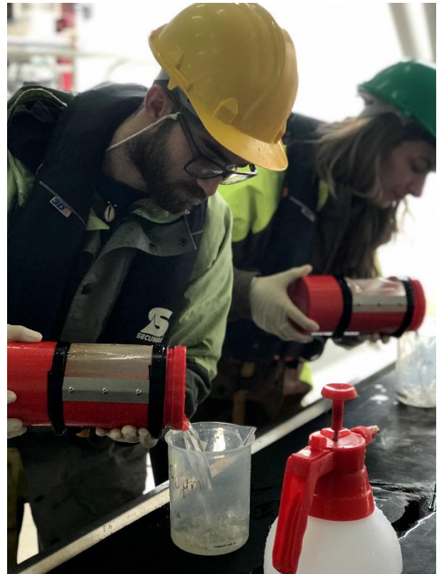
Figure 1.16 Bongo nets' cod-ends concentrate the plankton samples, which will be successively analysed for taxonomic identifications and for the examination of the chemical and biological properties of the plankton (photo taken by Sina Wallschuss).
