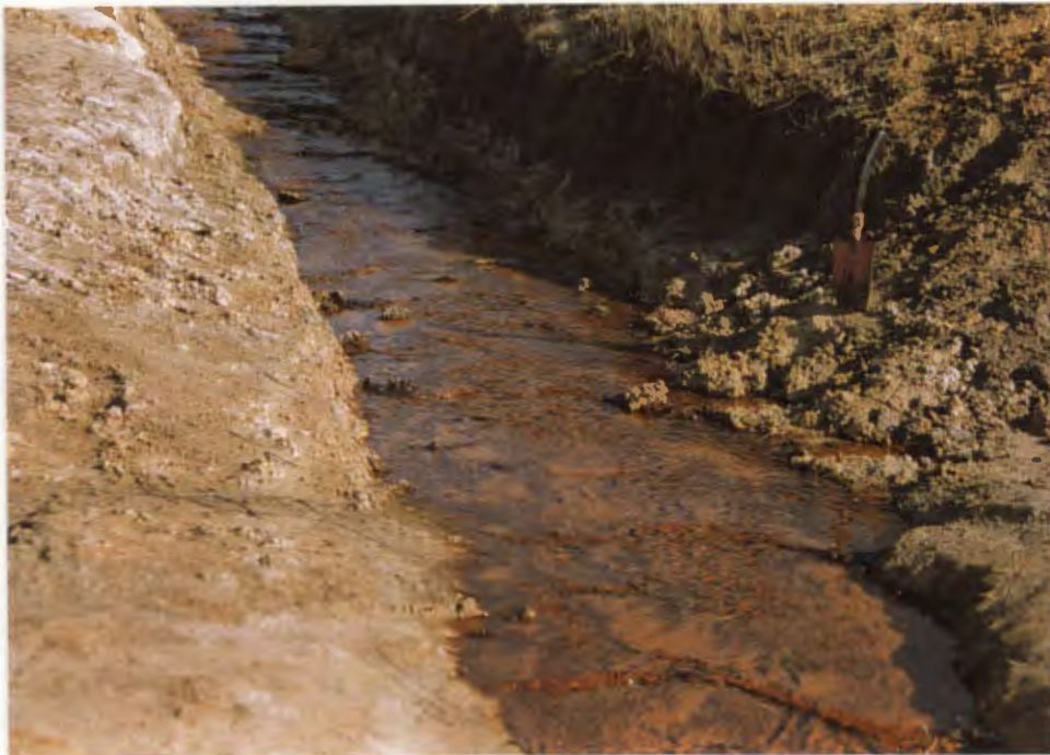
Figure 4.2 (continued) (C) Acid mine drainage dams immediately east of the seepage area (W5, W6) collect AMD from the seepage area and were overflowing. Drainage ditch (W9) redirected excess flow from the seepage area directly into the Blesbokspruit. (D) Acid mine drainage ditch (W15) with red-brown precipitate clearly visible.
