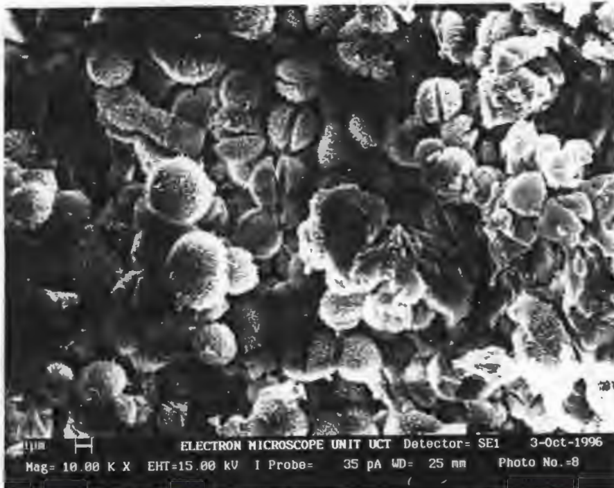
Figure 6.6 Scanning electron micrograph of precipitate P15 depicting spherical pincushion type crystal morphology. Bar = 1 \mu\text{m}
