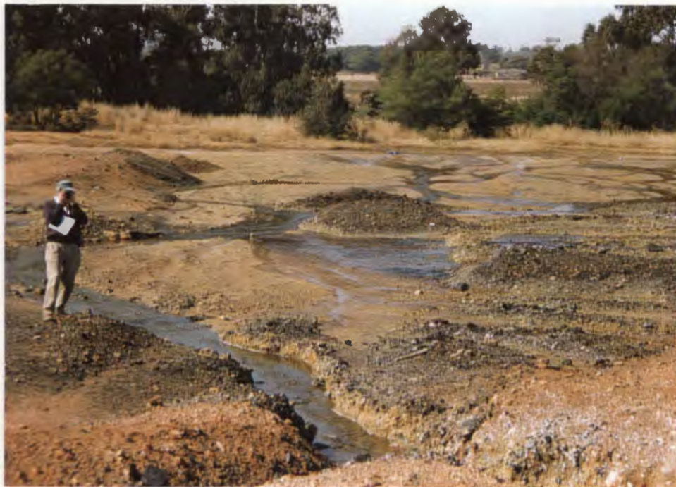
Figure 4.2 (A) The AMD outwelling point (W2), and (B) the seepage area on the west side of the Blesbokspruit. Algae growth and mineral precipitates are visible at both sites. Water seeps from the outwelling point and smaller seepage points along the ridgeline through the seepage area, collects and passes V-notch 14 before entering drainage ditch (W9).
