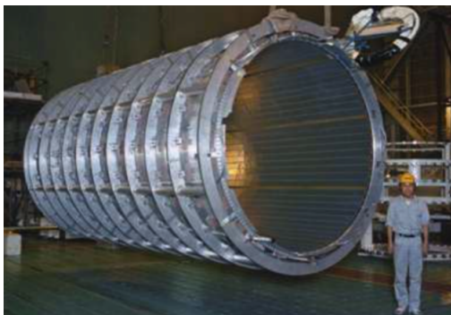
FIGURE 3.6: One of the solenoid magnets used in the ATLAS detector. The person can be used for scale [66].
