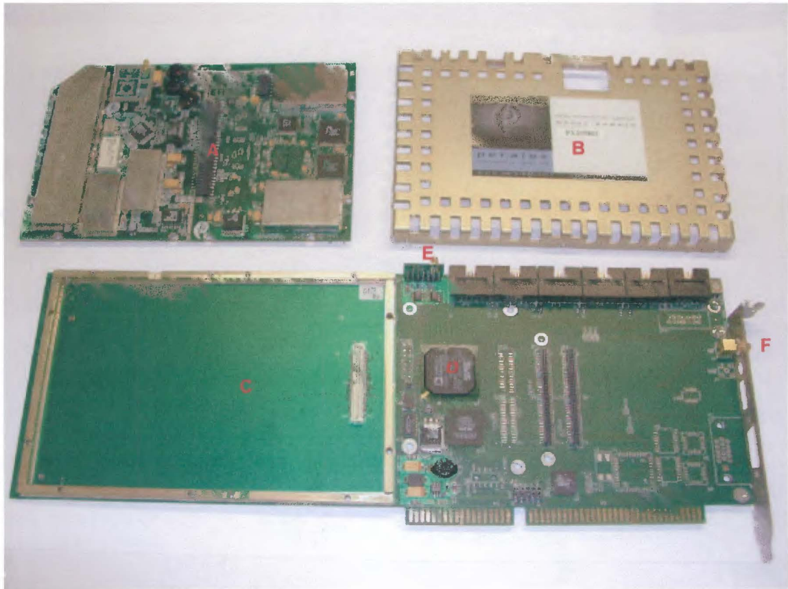
Figure D.3: Physical layout of the digital receiver adapter card and mezzanine module.
