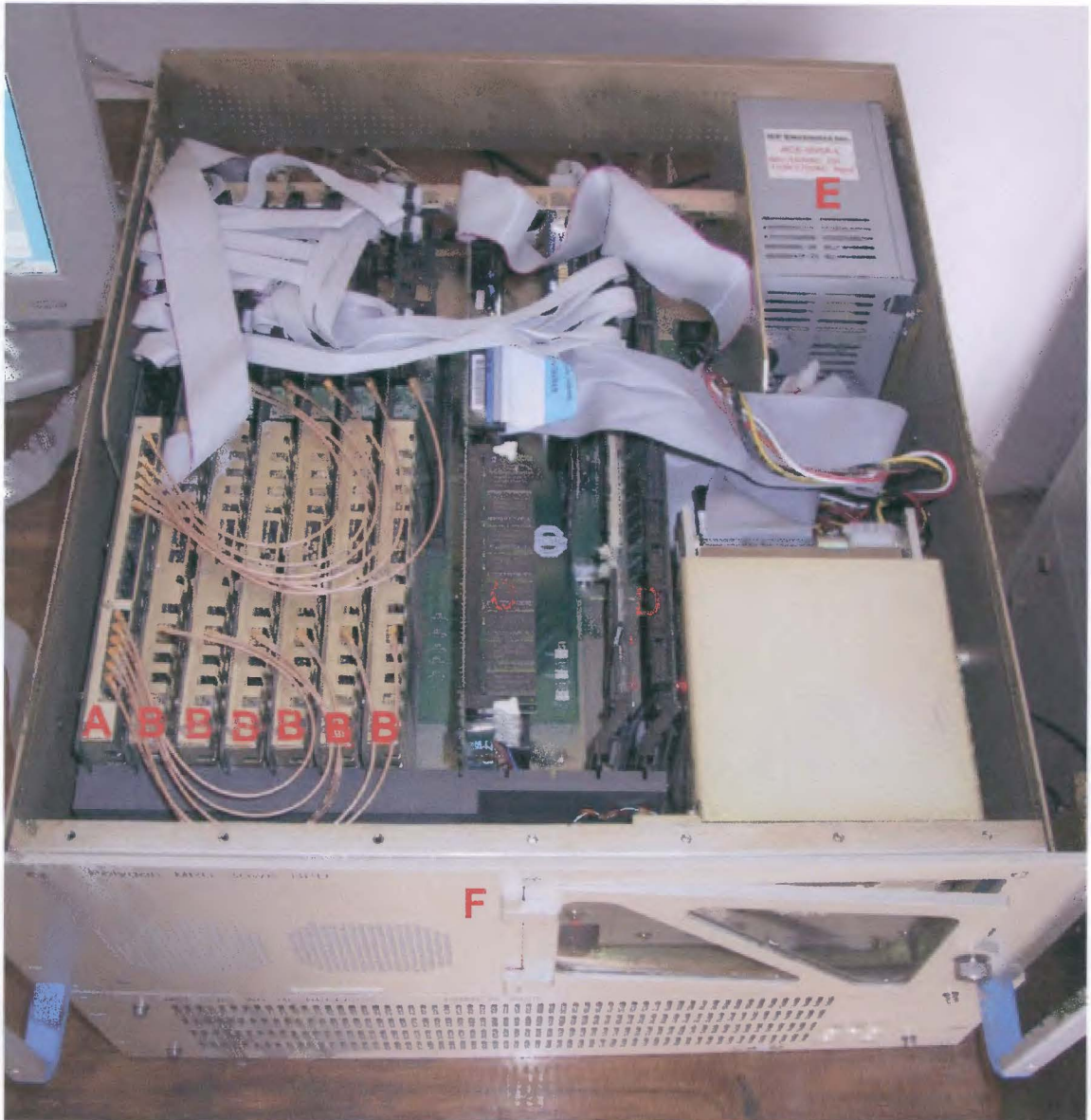
Figure D.2: 6-Channel wideband digital receiver.
