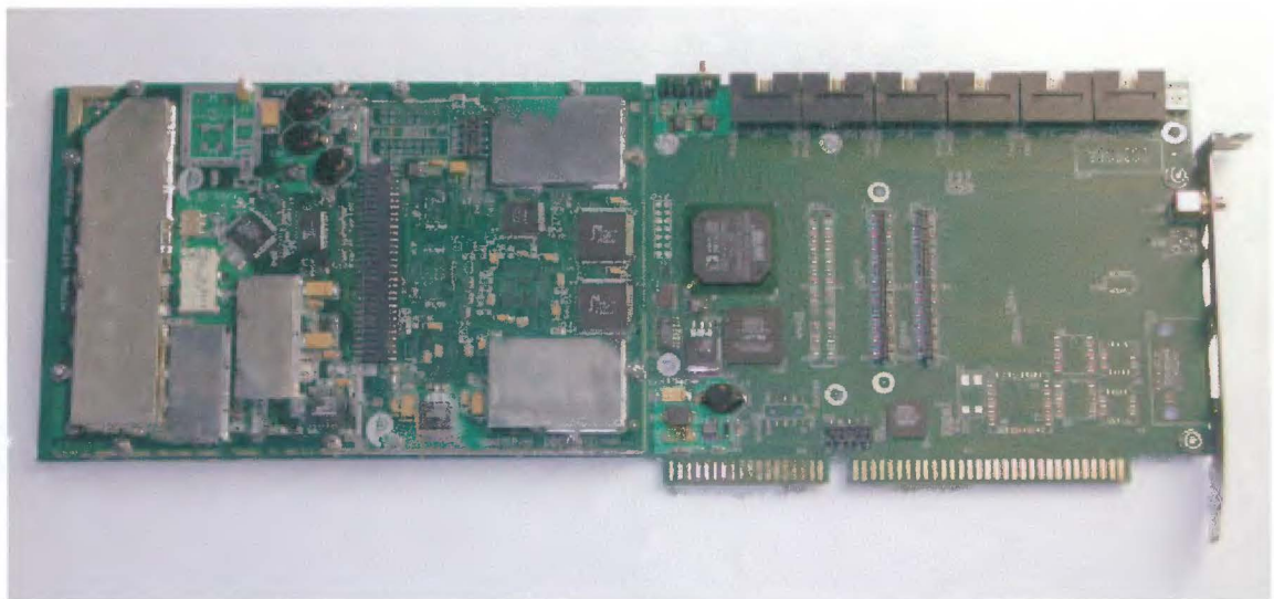
Figure D.5: Assembled digital receiver card (no shielding cover).
