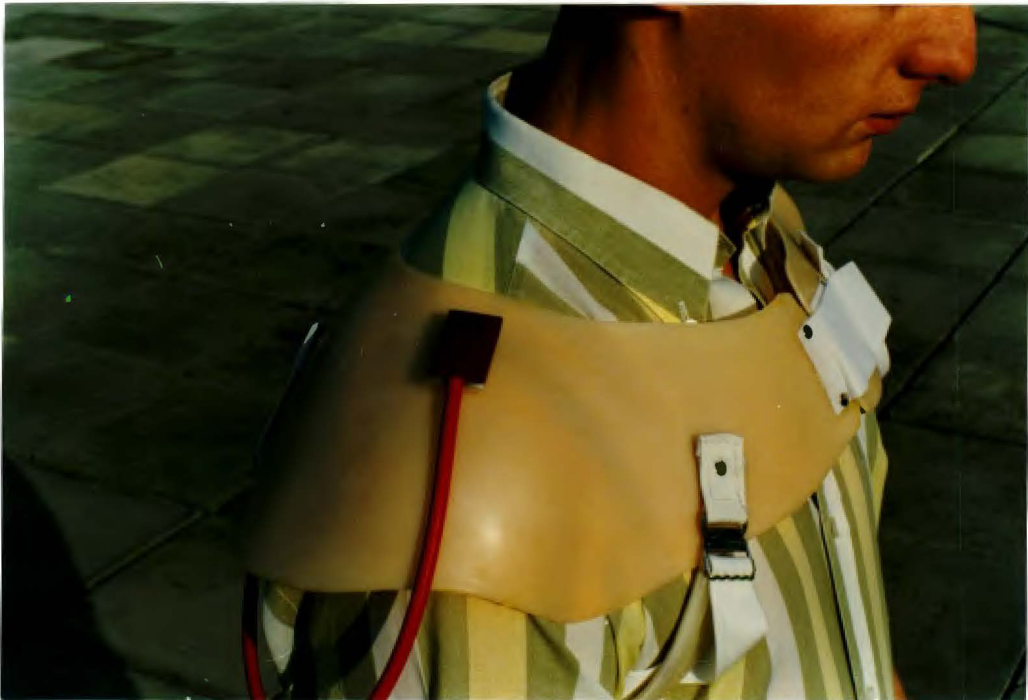
Fig 7.2 : Prototype shoulder pressure transducer
