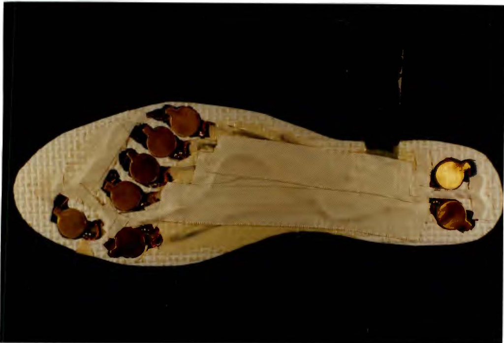
Fig 2.14 : Exposed insole showing transducer mounting
