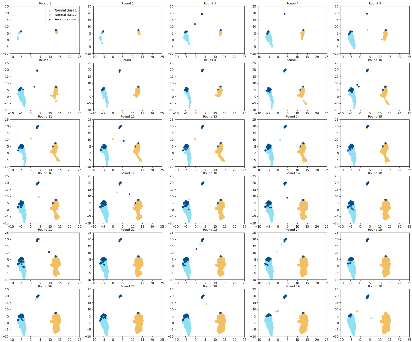
Figure A1.1: UMAP reductions for 30 rounds of training. In each round, there is a gradual separation of the anomalies (indicated in the deep blue dots) from the normal classes. This goes on until round 30 where the anomalies form a cluster and are completely separated from one of the normal classes (indicated in beige). It is also worth noting that, by round 30, there were fewer anomalies tightly coupled with the light blue dots (the other normal). A greater separation of the classes in the latent space indicates a separation of features which in turn helps with identifying anomalies.
