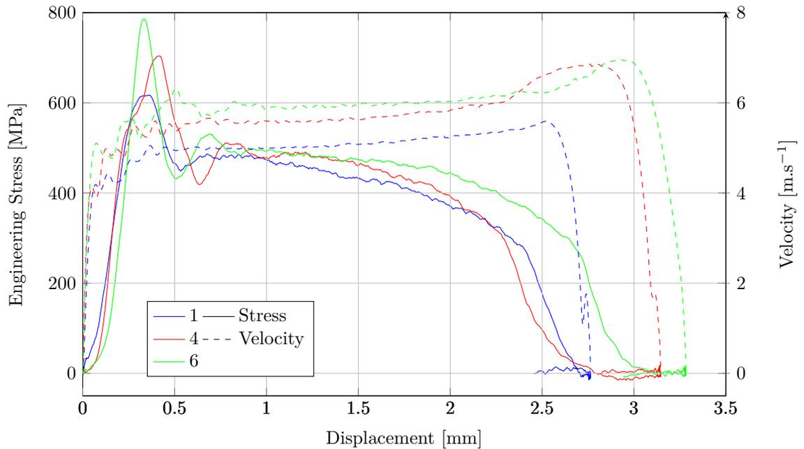
Figure 5.9: The deformation velocity is measured as the difference between the bar velocities on either side of the specimen.
