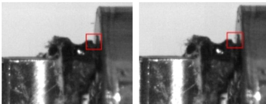
Figure 5.4: High speed camera images showing the threaded bar move within the output bar. The displacement can be seen by considering the tip of a thread as highlighted.
