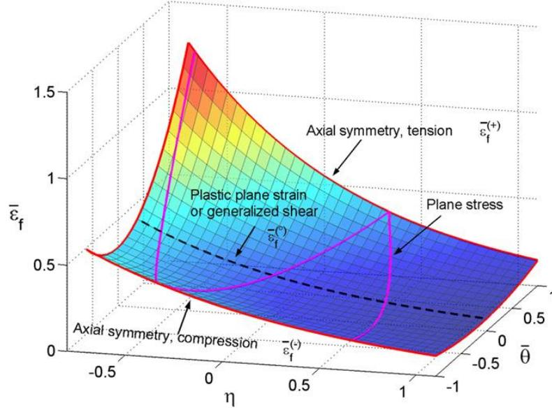
Figure 2.10: Fracture locus for the Bai-Wierzbicki damage model [17].
