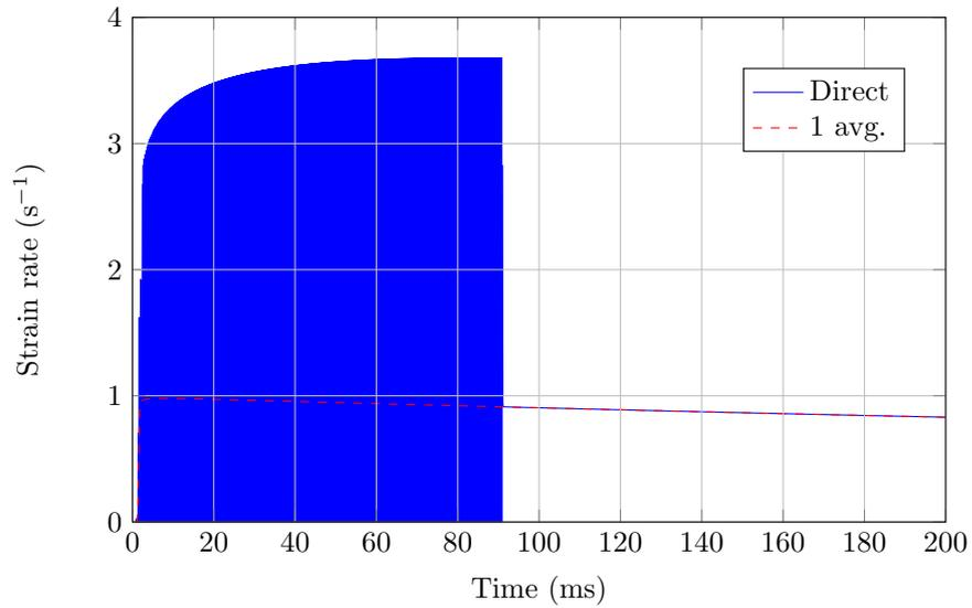
Figure 4.7: Strain rate of a single element test using a Predictor Return algorithm for the Zhao model at  $\dot{\epsilon} \approx 1$ . Using an average strain rate averaged over the previous and current step results in stability.
