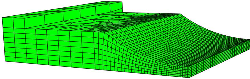
Figure 6.2: Quasistatic 5mm radius grooved specimen mesh.
