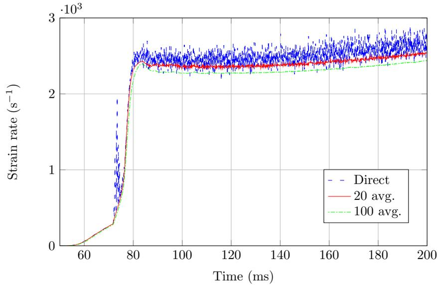
Figure 4.5: Strain rate resulting from using the Newton’s Method solver to simulate a SHB experiment. A weighted average is used to reduce oscillations.
