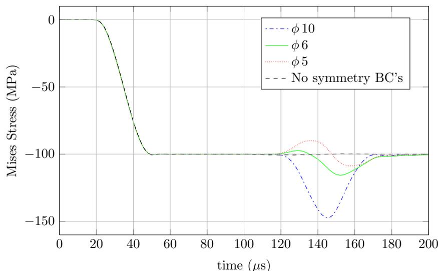
Figure 4.11: Effect of using circular beam elements with dimensions  $\phi 10$ ,  $\phi 6$  and  $\phi 5$ mm with a  $\phi 20$ ,  $\frac{1}{4}$  symmetry bar.  $\phi 10$ mm corresponds to the same cross-sectional area as the bar. Also shown is the result from using a full 3D bar, with no symmetry boundary conditions, together with beam elements of the same dimensions.
