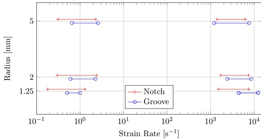
Figure 6.12: Initial and final strain rate of the element in the centre of the specimen. The final strain rate is similar across all the different specimens for both those deformed dynamically and at quasistatic rates.
