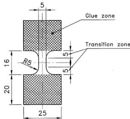
Figure 2.26: Tensile sheet specimen design used by Verleysen and Degrieck [36].
