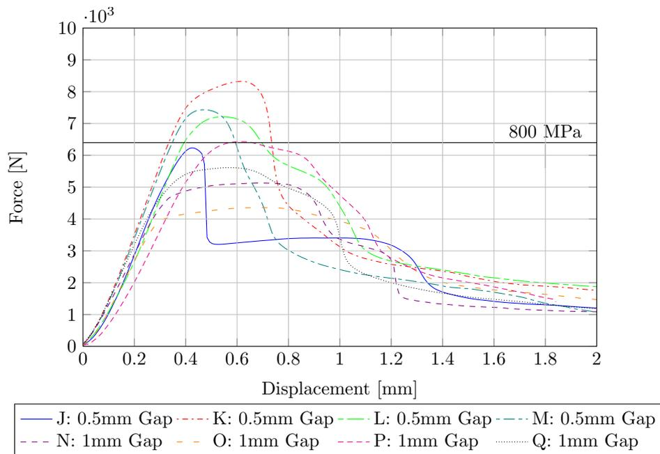
Figure 3.14: Results from Glue Test set 2 showing pulling force versus displacement. The cut-off line indicates the force required to reach a stress of 800MPa in a specimen of gauge section  $4 \times 2$  mm.
