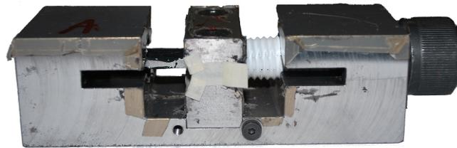
Figure 3.20: Bar bonding to specimen in the jig. The cap screw aligns the rear of the bar and compresses it against the clamp.
