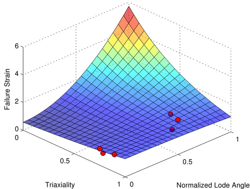
Figure 6.19: Fracture locus generated using the dynamic results.
