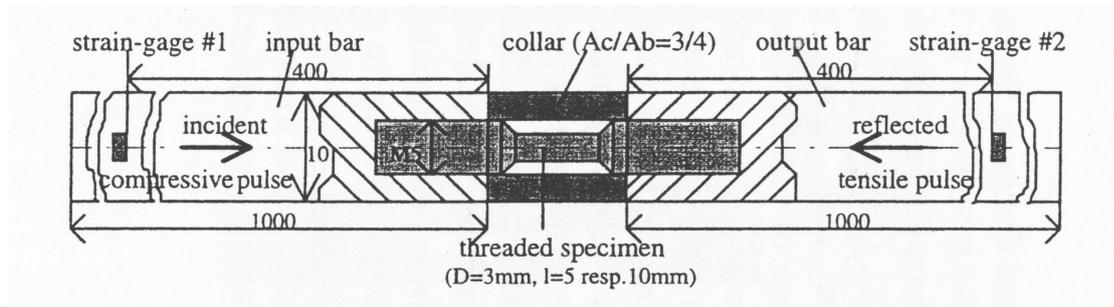
Figure 2.16: Modified compression bar as used by Nicholas [32].
