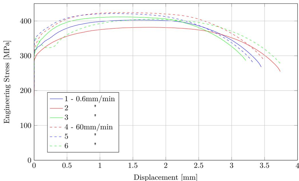
Figure 5.8: Quasistatic results for the straight specimens.
