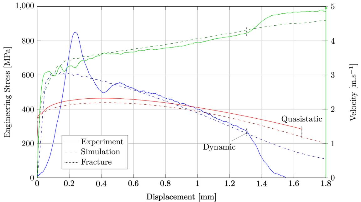
Figure 6.6: Simulation of the 2mm radius notched specimen compared to the experimental result.
