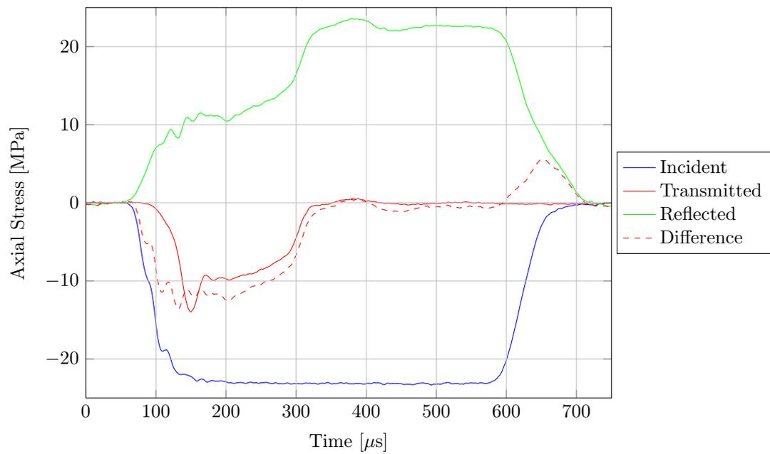
Figure 5.33: Strain gauge readings for 2mm radius grooved specimen 3.
