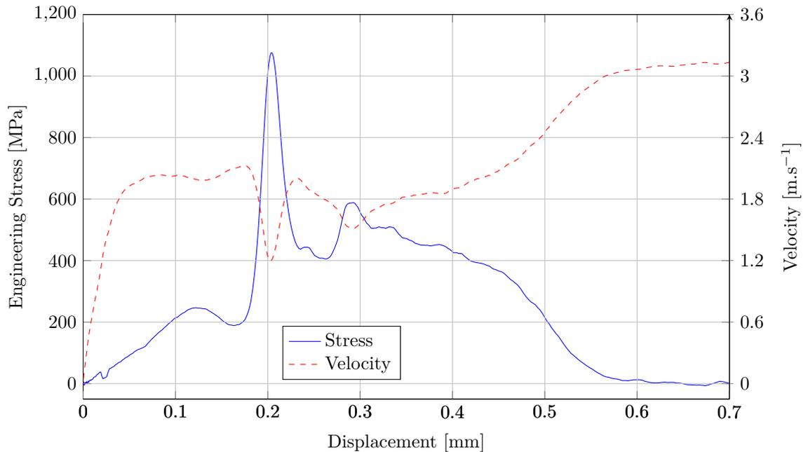
Figure 5.5: TSHB results for the 2mm radius grooved specimen 2.
