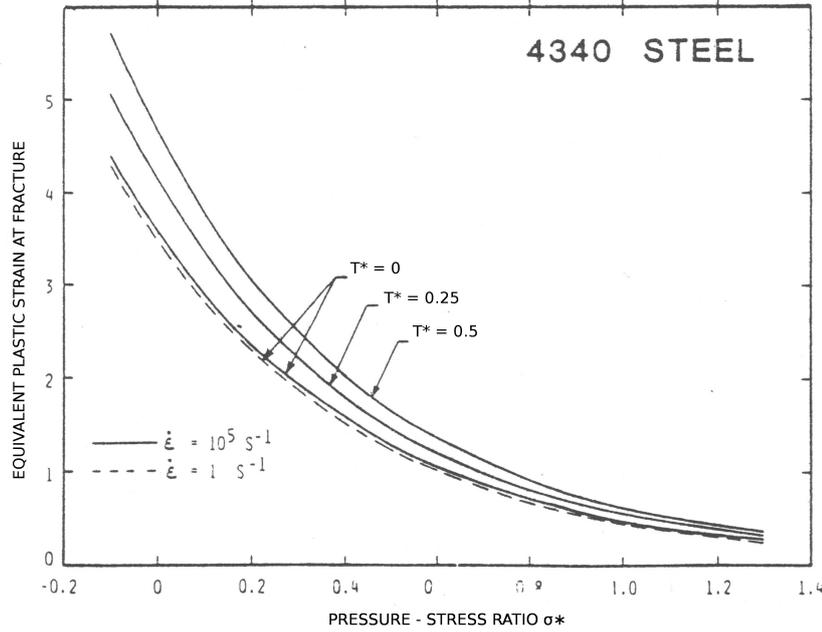
Figure 2.3: Johnson-Cook fracture model for 4340 Steel[14].
