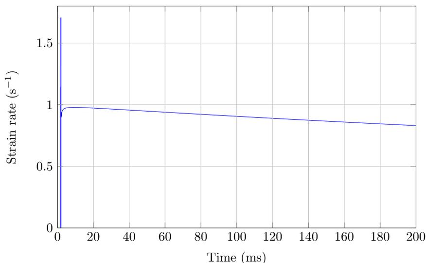
Figure 4.6: Strain rate of a single element test using a Predictor Return algorithm for the Johnson Cook model
