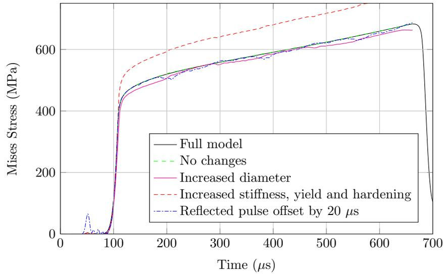
Figure 4.12: Specimen stress versus strain curves resulting from using velocity boundary conditions. The full model is compared to that using the velocity BC's with the same specimen properties. The properties are then changed resulting in poor correlation.
