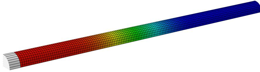
Figure 4.13: Model used to study the effect of placing infinite elements in place of the input bar. The infinite elements are in the foreground.
