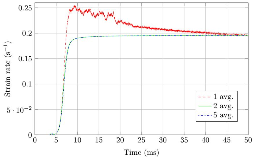
Figure 4.8: Strain rate of a single element test using a Predictor Return algorithm for the Zhao model at a slow strain rate of 0.2. In this case a weighted average of  $N = 2$  is required for stability
