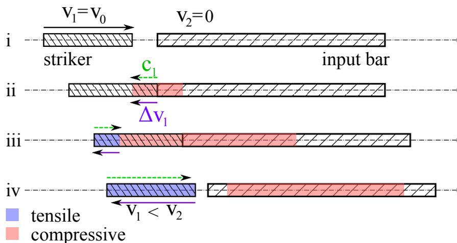
Figure A.3: Impact of the striker and incident bars.  $c_1$  indicates the direction of the wave, while  $\Delta v_1$  considers the change in particle velocity through the striker.
