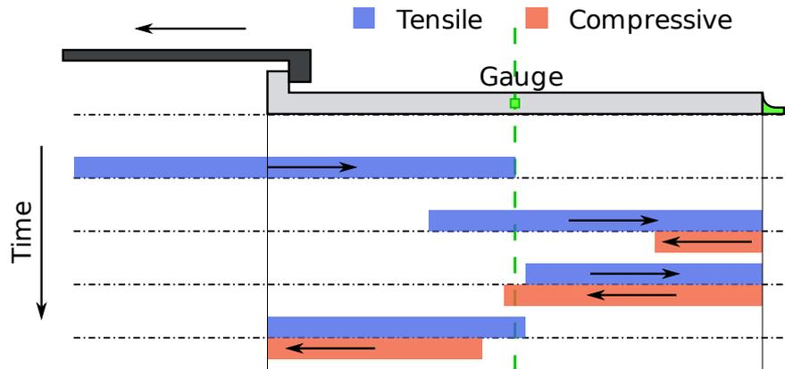
Figure 3.5: Stress wave propagation through the input bar.
