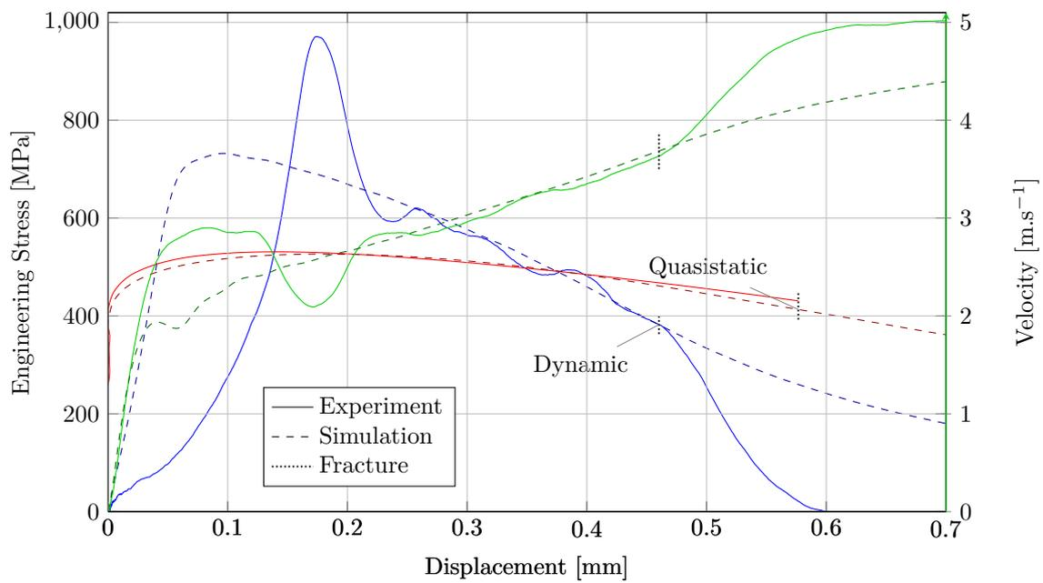
Figure 6.8: Simulation of the 1.25mm radius grooved specimen compared to the experimental result.
