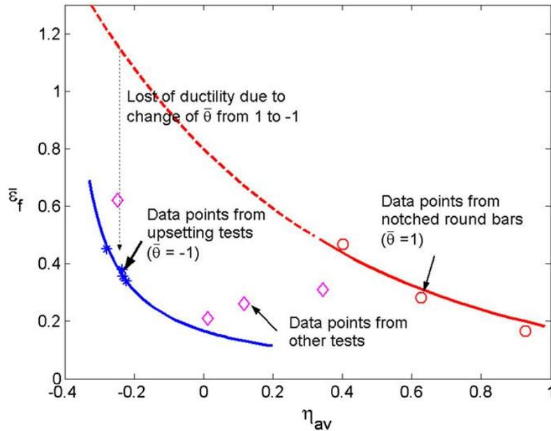
Figure 2.9: Ductility change between  $\bar{\theta} = -1$  and 1 [17].
