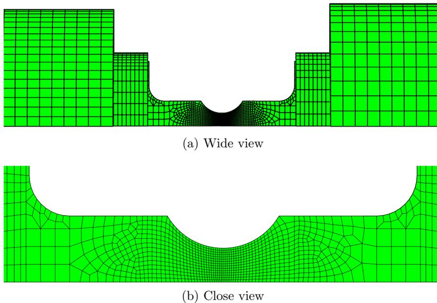
Figure 6.1: Dynamic 2mm radius notched specimen mesh.
