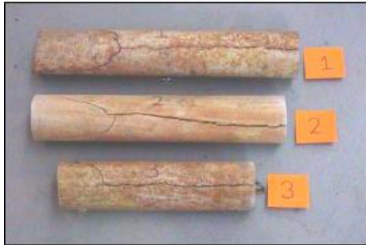
Figure 5-79: Typical failure mechanisms in AC pipes ( Greyvenstein & van Zyl, 2005)
