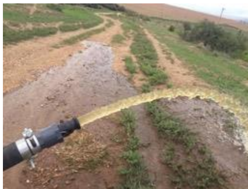
Figure 5-51: Showing the colour of water during the flushing process of the BS8 pipeline test 1 pipeline
