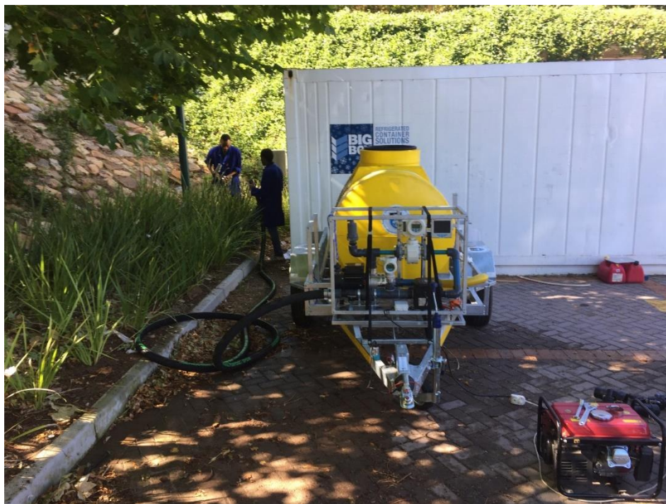
Figure 3-20: Constructed pipe condition assessment equipment (PCAE) outside the laboratory at the University of Cape Town
