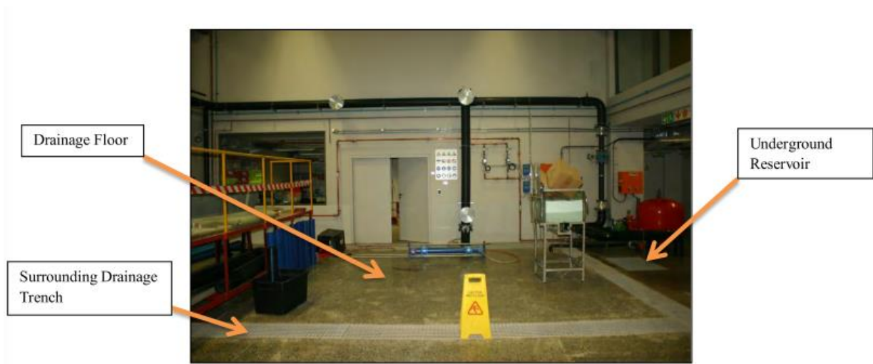
Figure 4-1: Picture of the hydraulic section of the Civil Engineering Laboratory at the University of Cape Town (Malde & van Zyl, 2015)
