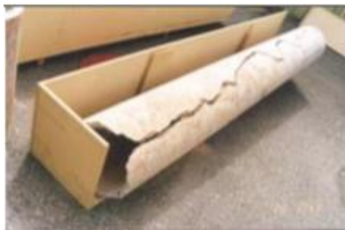
Figure 2-51: Failure mode of an AC pipe: longitudinal split
