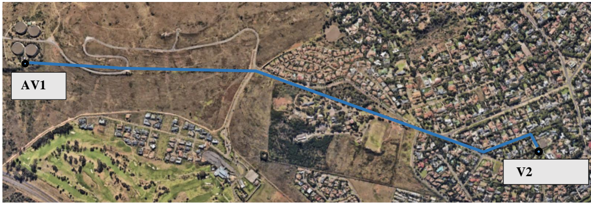
Figure 5-33: Map showing FC pipeline route starting at AV1 (5bar+) and ending at V2 0.3 bar+)
