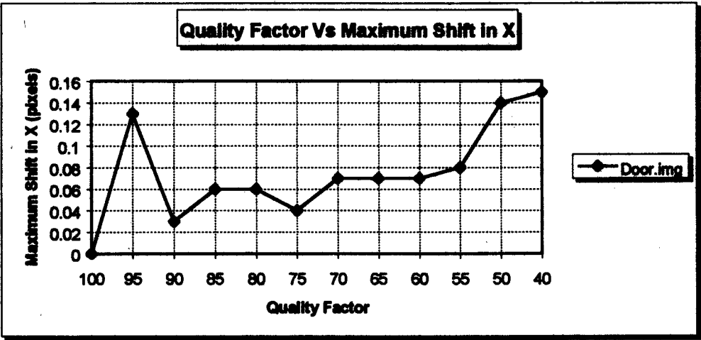
FIG 5.19: Quality Factor Versus Maximum Shift in X for door image using JPEG (DCT-based) Compression
