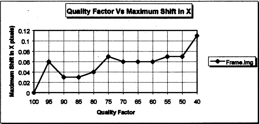
FIG 5.13: Quality Factor Versus Maximum Shift in X for frame image using JPEG (DCT-based) Compression
