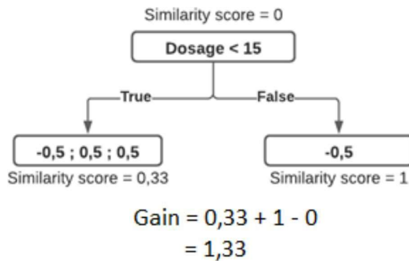
Figure 15. Example of a branch of an XGBoost decision tree showing the similarity scores used to calculate gain
