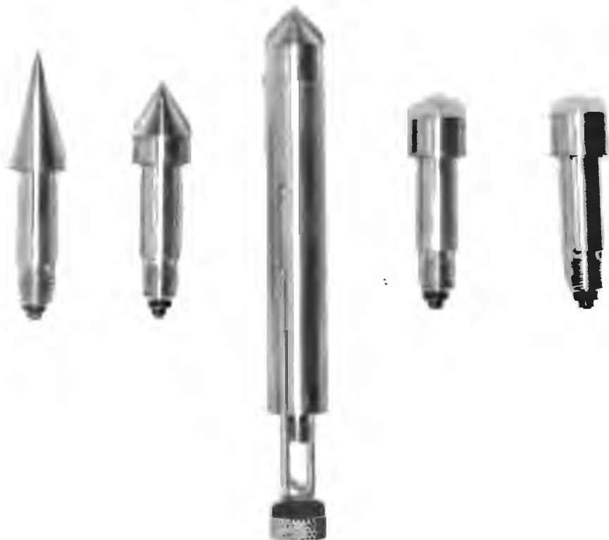
Photo 5.6 The projectile used to monitor inner zone radial expansion and its range of segmented heads. Note the partially inserted commutator wire.
