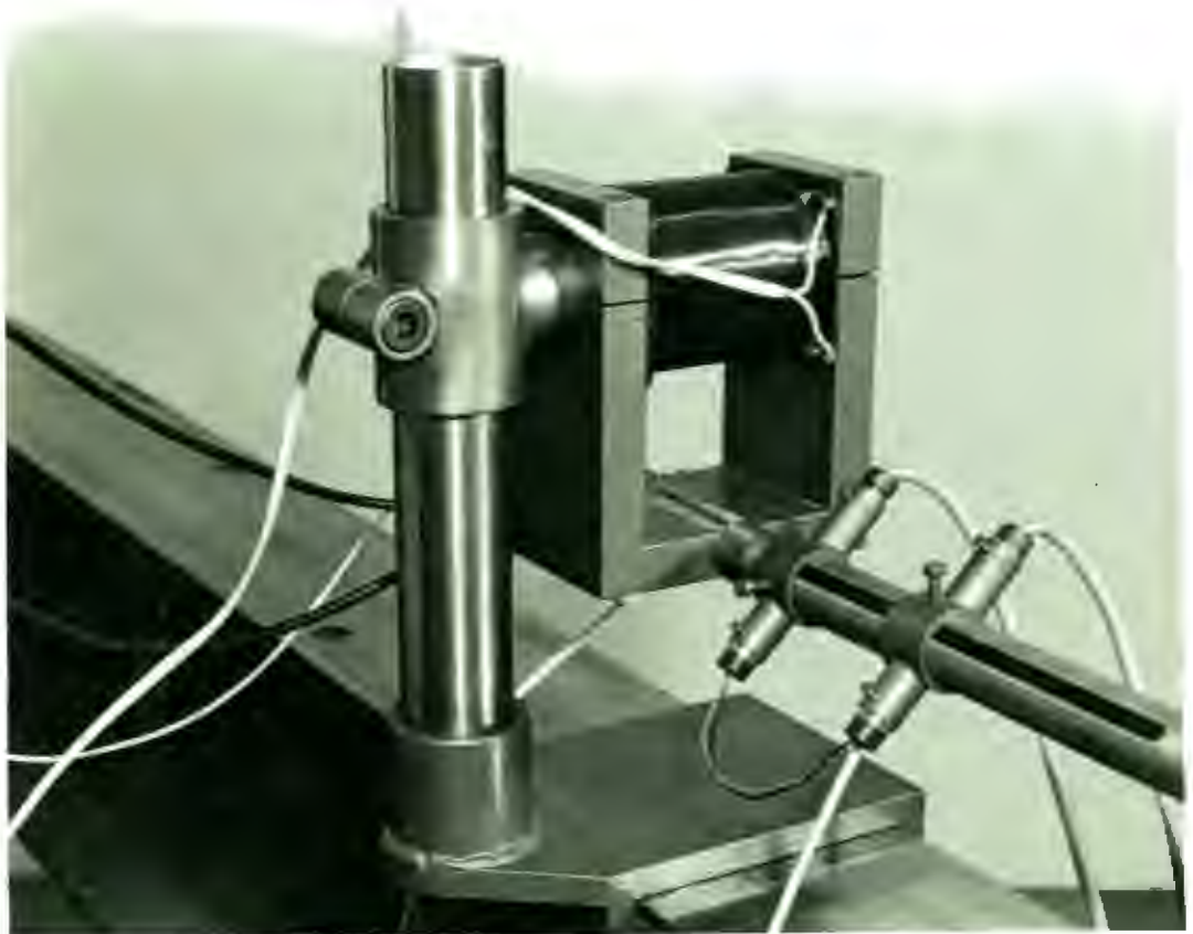
Photo 5.2 Rear view of the field magnet showing the slotted section of gun barrel and the photo-electric device used to measure the projectile approach velocity.
