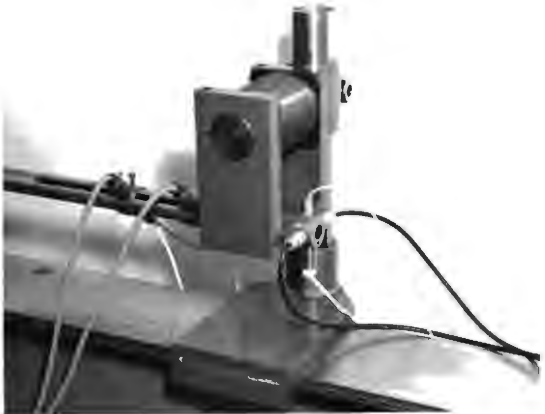
Photo 5.4 The field magnet and pickup section showing the scratch pickups and photo-electric pulse generator.
