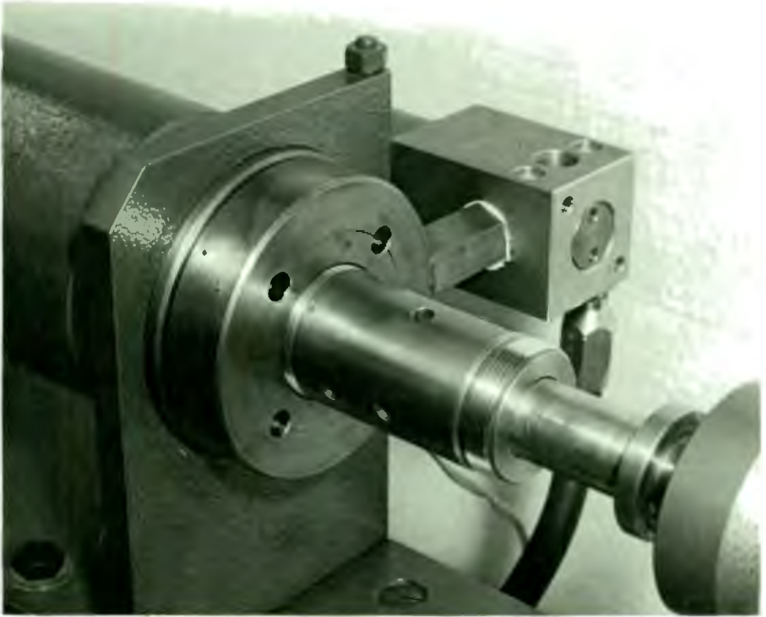
Photo A.3 The breach of the gas gun showing the triggering solenoid
