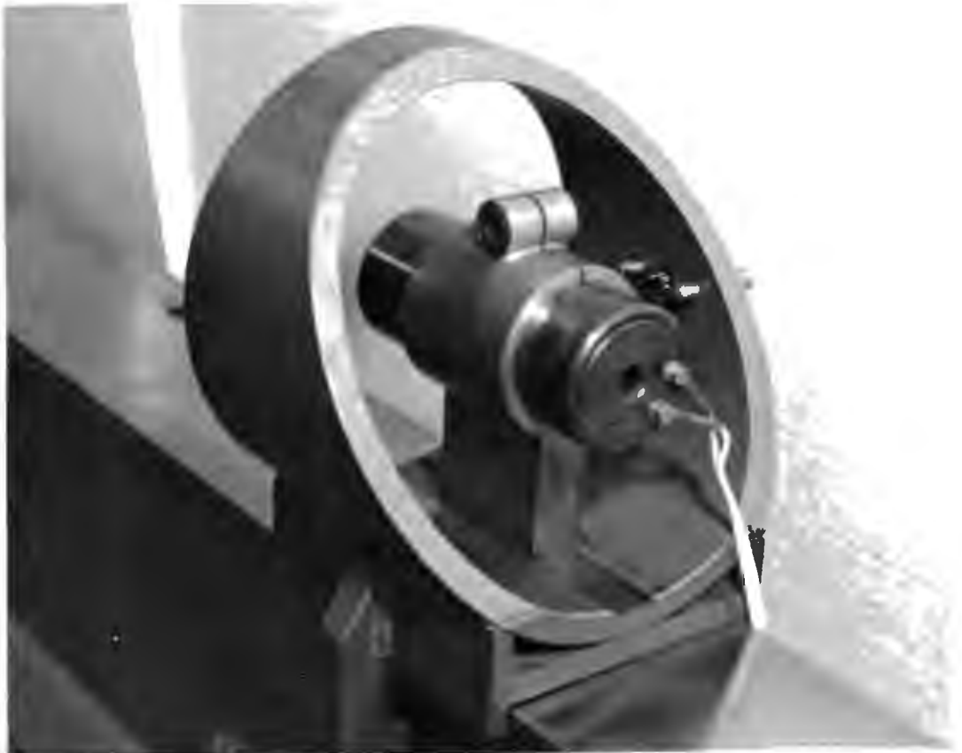
Photo 5.8 Rear view of the target transducer field magnet and mounting
