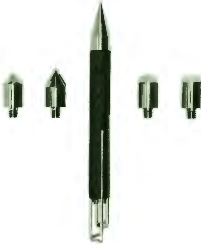
Photo 5.1 The force monitoring projectile with its range of heads. Note the partially inserted commutator wires.
