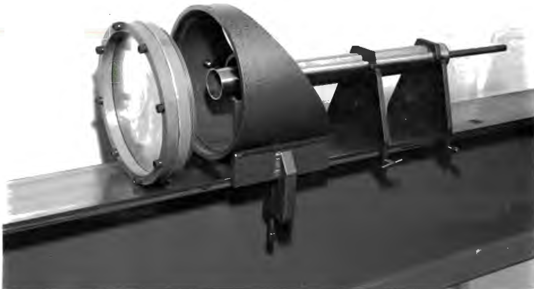
Photo A.2 The target mounting and projectile catcher
