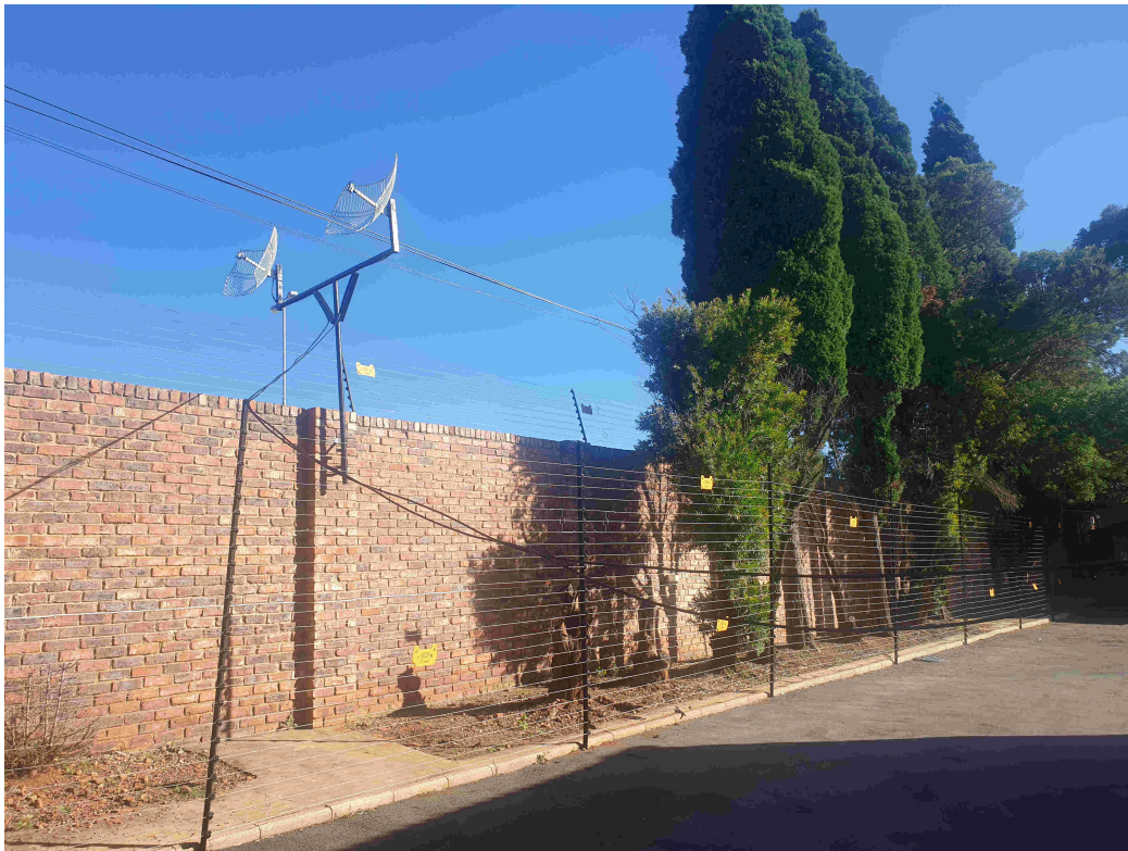
Figure 5.15: Antenna Deployed For Airborne Targets Detection
