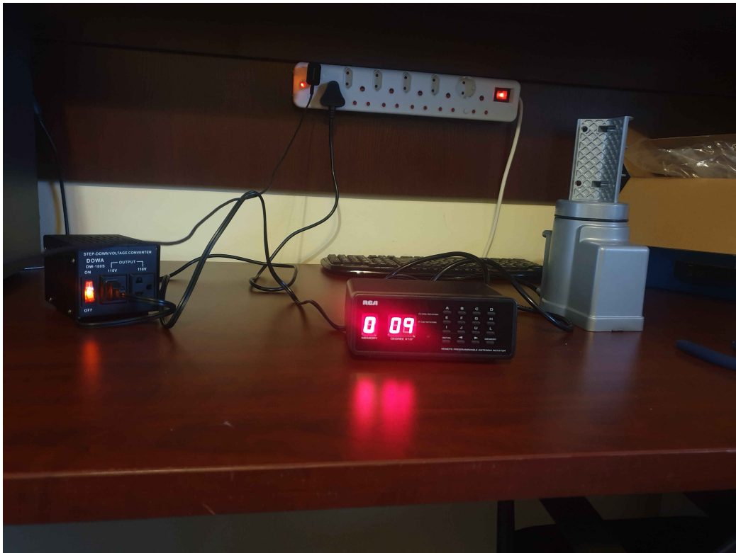
Figure 5.22: Antenna Rotator Before Installation
