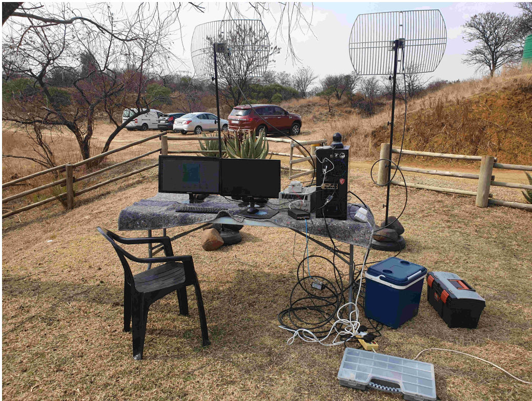
Figure 5.25: Radar Setup For Airborne Targets Detection Phase 3
