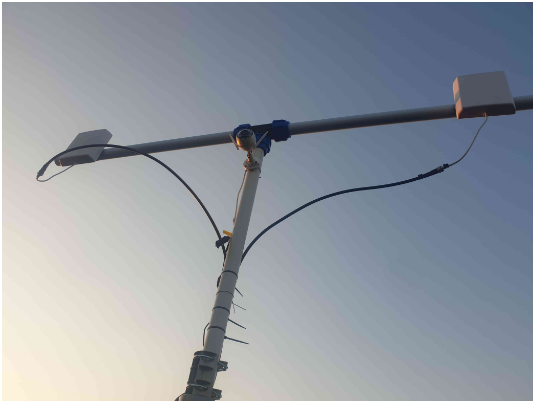
Figure 5.20: Antennas, T Mast, Camera And Rotator Deployed For Airborne Targets Detection Phase 2
