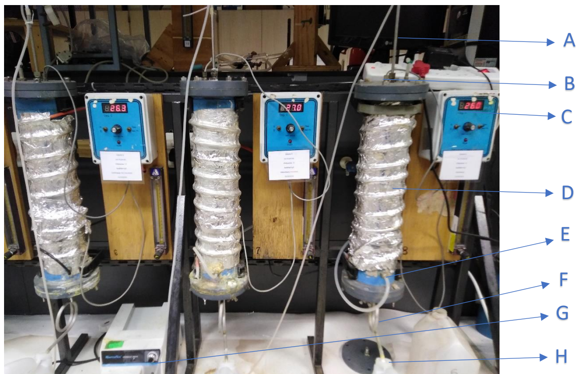
Figure 3-2: Bioleach column reactor system. A (feeding inlet), B (inside temperature sensor), C (temperature control unit), D (outside temperature sensor), E (air inlet), G (pump) and H (collection of leachates)
