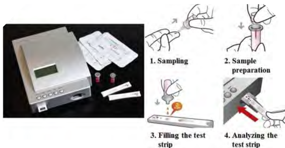
Figure 1-9: The i-CHROMA POC CRP test. The device automatically calculates and presents CRP results for concentrations ranging from 2.5mg/L to 300mg/L 84
