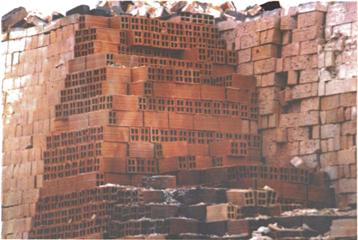
Hollow blocks fired in a clamp at Claytile (Pty) Ltd, Koelenhof in February 1993. The distorted blocks can be seen in the right foreground.
