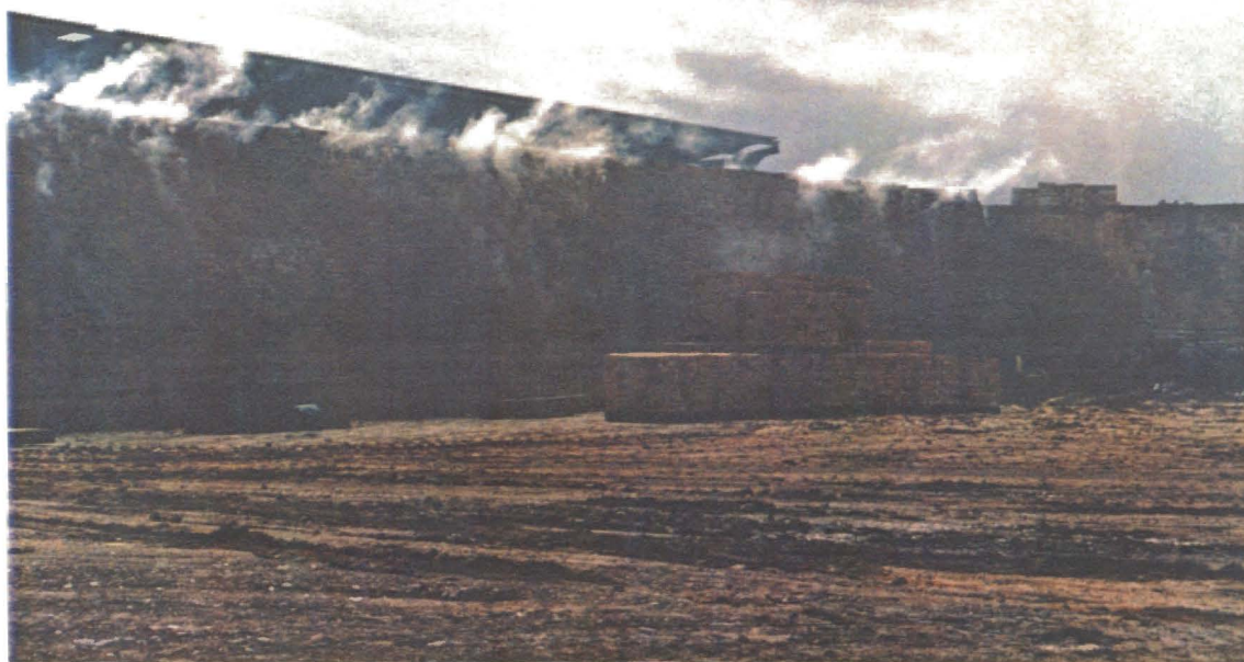
A clamp which is burning at Joostenberg Brick.
