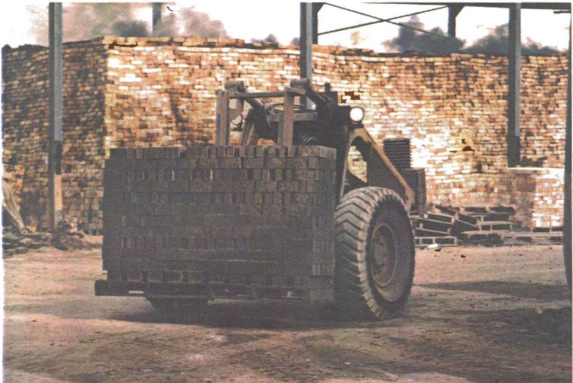
A Bell FL220 forklift transporting a wooden pallet with a with bricks stacked in the "Hulo" configuration
