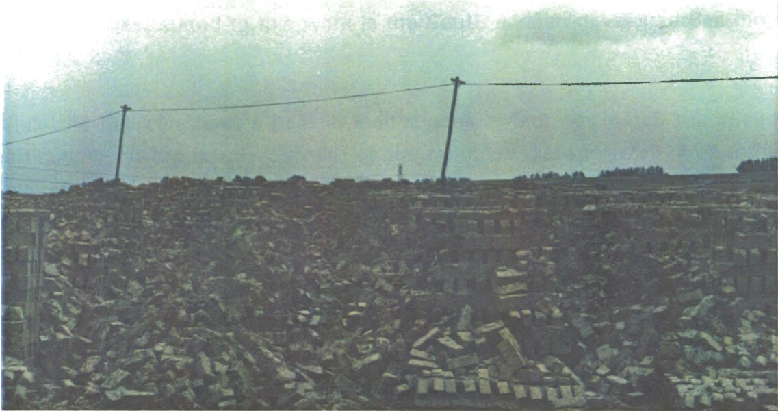
Square pallets, at Claytile in Koelenhof ,these bricks had been made and set on the day before the rain
