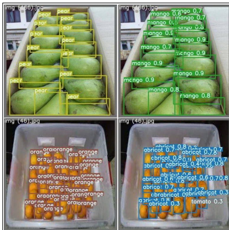
Figure 18: Comparison of actual labels (left) and YOLOv71 predictions (right): the model successfully identified the presence of objects of interest and their spatial locations within the image. But, it struggled to accurately determine their categories due to their similarity and partial obscuration.
