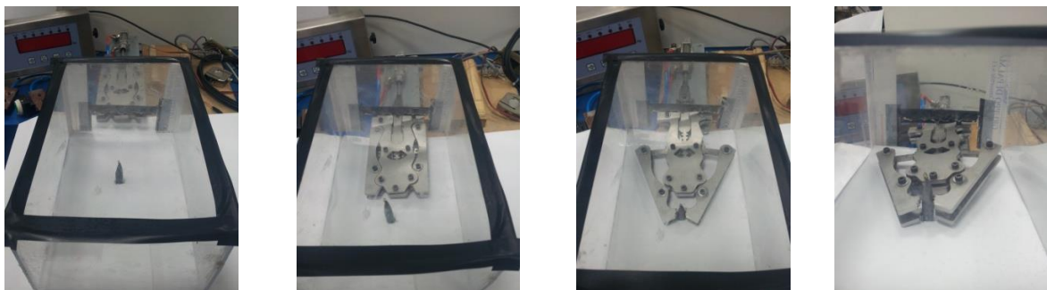
Fig. 1: Gripping operation of an object inside an enclosure communicated with the exterior via an opening.
