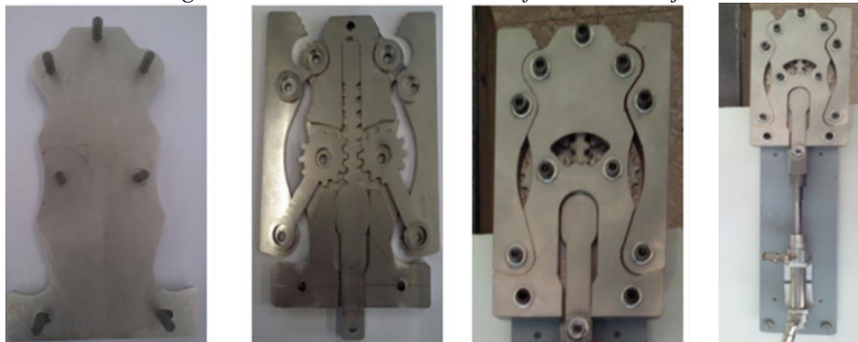
Fig. 5: Model of the retractable two finger gripper in stainless steel
