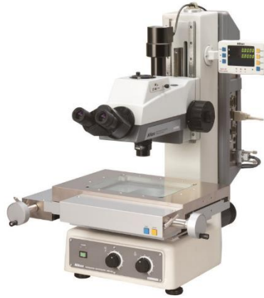
Figure 4.4: OM apparatus used in the present work (MM-400, Nikon).
