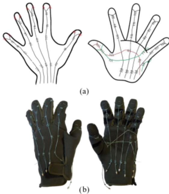
Fig. 1. (a) Attachment points between the tendons and the glove: left side for the flexion movement, right side for the extension movement. (b) Tendon routing over the soft exo-glove: for the flexion movement - right side and for the extension movement - left side.
