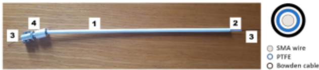
Fig. 3. SMA-based actuator-left side (1-Bowden Cable, 2-PTFE Tube, 3-SMA Wire, 4-Terminal Unit); Actuator schematic concept -right side.
