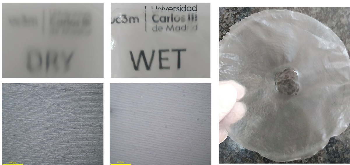
Fig. 12 Macroscopic (top) appearance of CA patterned films obtained on PTFE surface, in dry (left) and wet (right) state and micro-photograph of corresponding surfaces (bottom); circular translucent film with wetted central part showing difference in transparency
