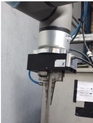
(b) Real gripper integrated in the robot.
