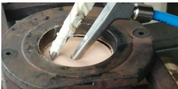
Fig. 12 Vacuum finger introduction
