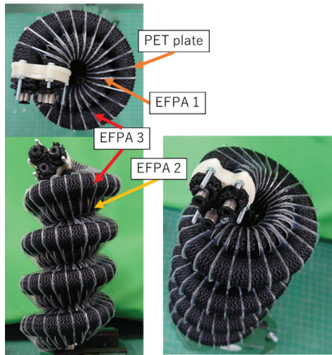
Fig. 4. Overview of spiral soft actuator with circumferential restrain mechanism.
