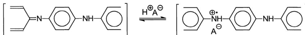
SCHEME 1 Scheme of the protonation of PANI base with acids. Adapted with permission. 32 Copyright 1998, American Chemical Society.
