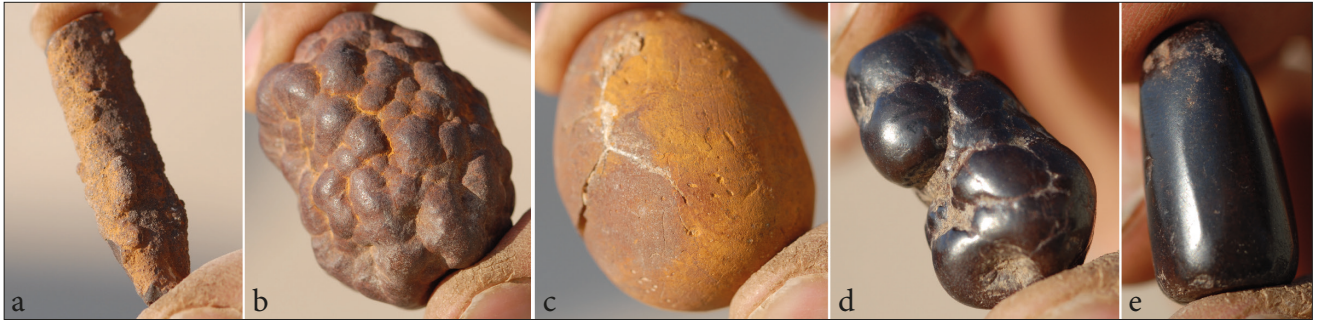
Fig. 4. Different stages of processing of goethite rock
