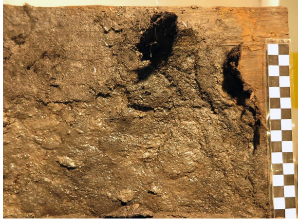
Fig. 7 Horse hair found between BV1's sheathing and hull planking (photographs by the authors)
