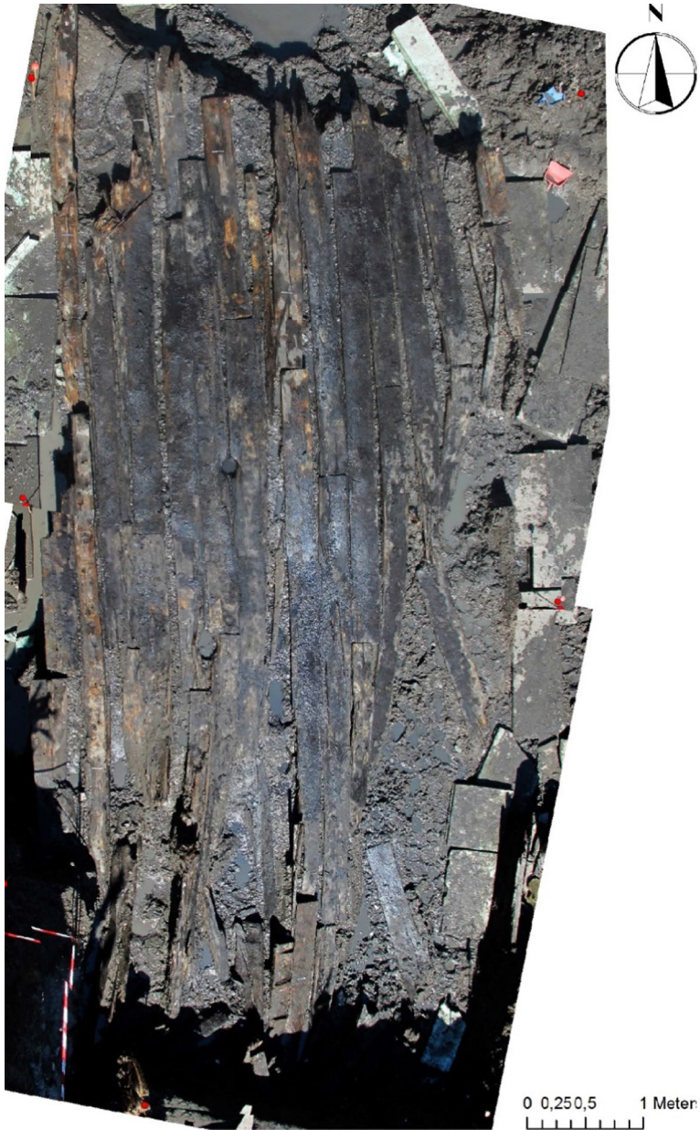
Fig. 4 The BV1 ship sheathing planks during the archaeological works (Photogrammetry: CHAM archives)
