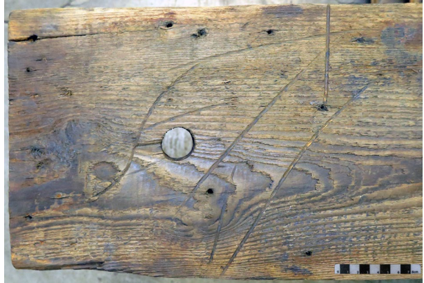
Fig. 5 Incised marking on inner face EDP_0247 sheathing plank (photographs by the authors)
