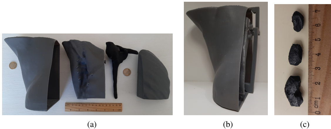
Figure 4.4: Physical phantom of the axillary region. (a) from left to right: 3D-printed torso, muscle, bone and lung are represented. Note that the torso, muscle, and lung compartments are hollow. (b) assembled phantom; a fixture which keeps the organs in place can be observed. (c) three solid ellipsoidal axillary lymph nodes made of rubber.
