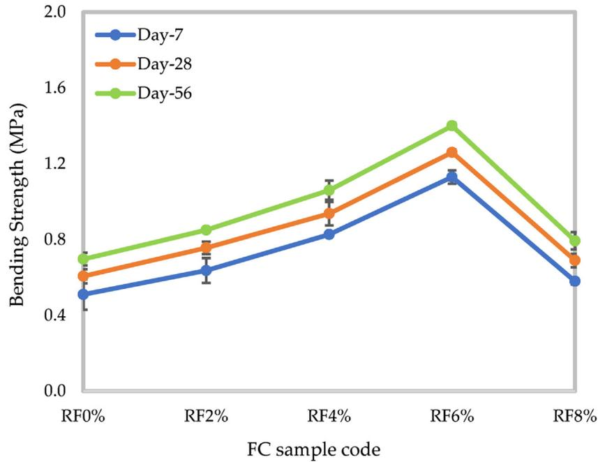
**Fig. 11 – Bending strength of FC-RF composites.**
