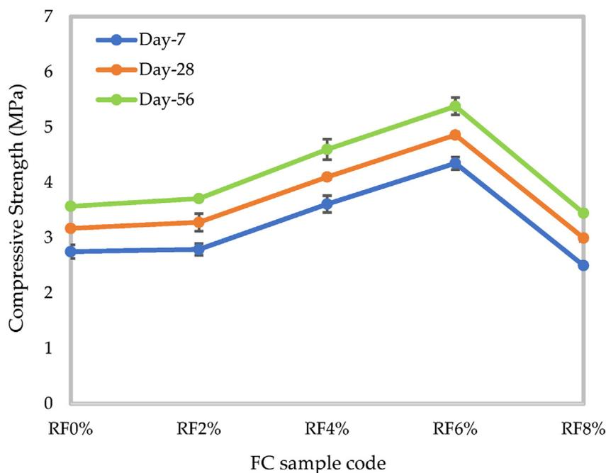
Fig. 10 – Compressive strength of FC-RF composites.
