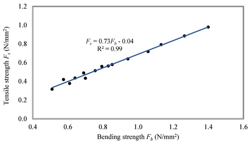
Fig. 14 – Relationship between FC-RF composites' bending-compressive strengths.
