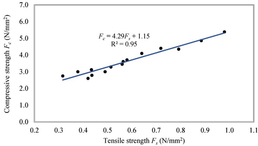
Fig. 15 – Relationship between FC-RF composites' tensile-compressive strengths.
