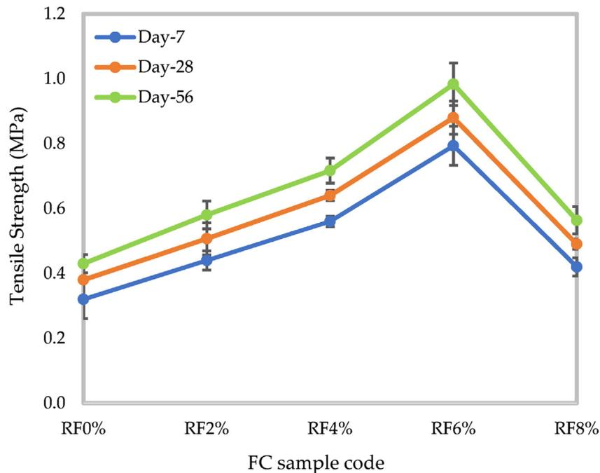
**Fig. 12 – Tensile strength of FC-RF composites.**
