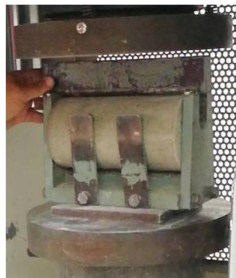
**Fig. 5 – The tensile test was accomplished on a 100 mm in diameter x 200 mm in height prism.**
