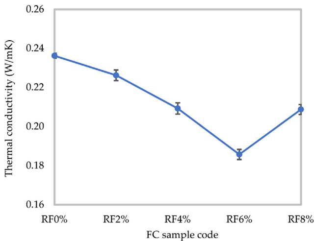
Fig. 17 – Thermal conductivity of FC-RF composites.
