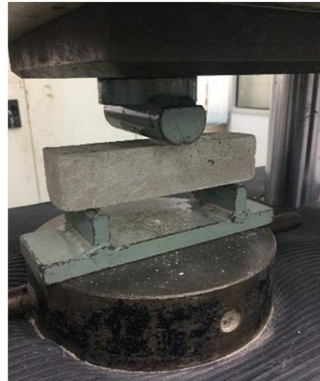
**Fig. 4 – The bending test was executed on a  $100 \times 100 \times 500$  mm prism.**
