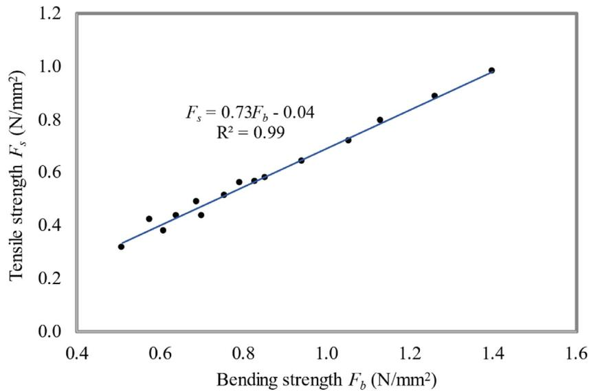
Fig. 16 – Relationship between FC-RF composites' bending-tensile strengths.
