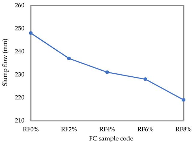
Fig. 7 – Slump flow of FC-RF composites.
