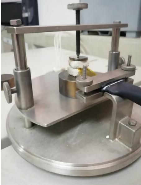
Fig. 6 – Setup for a thermal conductivity test.
