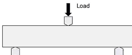
**Fig. 3 – Diagram of the three-point bending test arrangement.**
