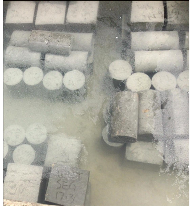
FIGURE 2: Curing of concrete samples in the water tank.
