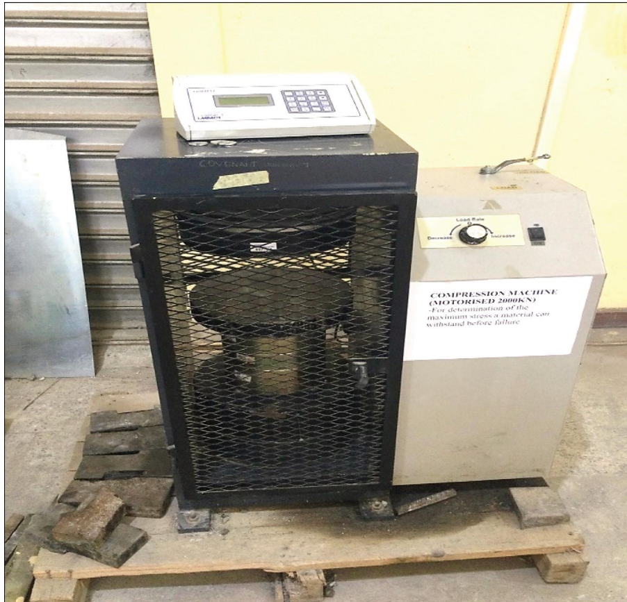
FIGURE 3: Compressive strength machine.
