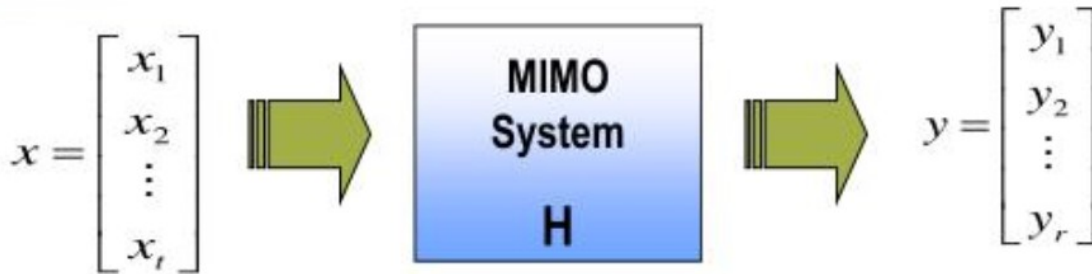
Fig. 1.13. The model of the MIMO system used to model the channel mathematically.
