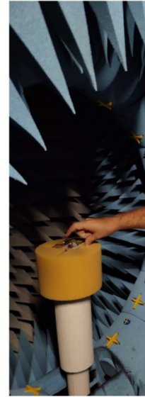
(b) The fabricated antenna in the chamber for measurements.
