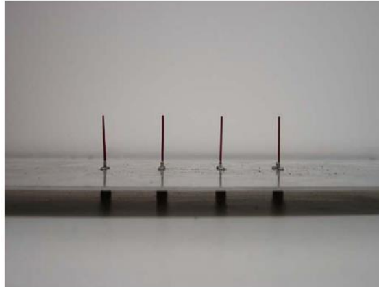
Figure 15 The four element monopoles array [30].
