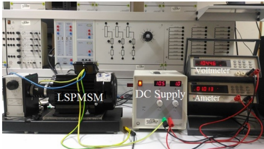
Figure 4.2 DC test setup
