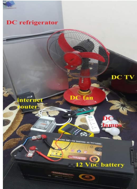
Figure 5.6: Experimental set up for DC-DC configuration (12 V DC appliances case)
