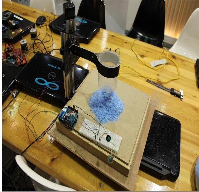
Figure 15: Angle of Repose Measurement Instrument
