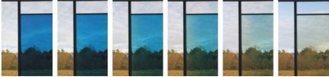
Figure 2.28 Switching sequence of an electrochromic laminated glass [108].
