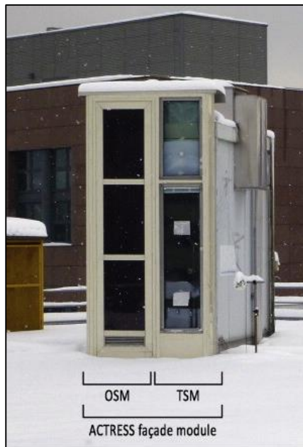
Figure 2.29 The developed ACTRESS MFM prototype [105].
