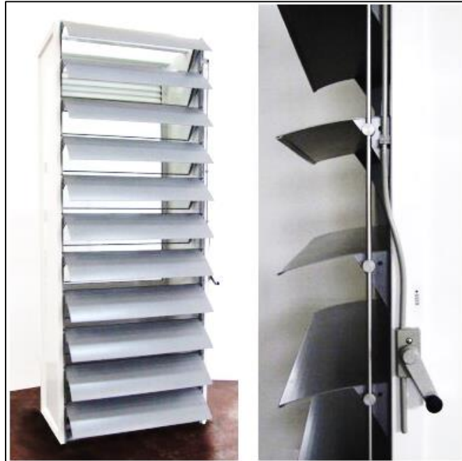
Figure 2.1 Prototype of the double skin façade proposed in an open configuration [24].
