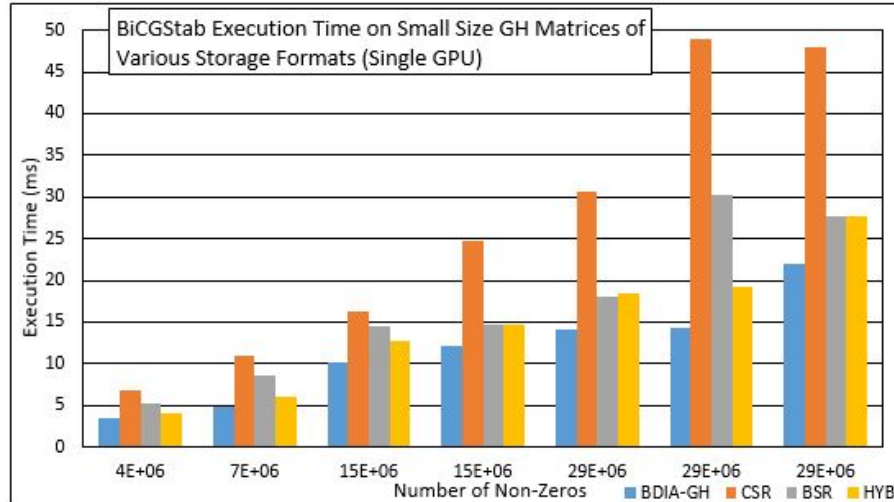
Figure 6.6: BiCGStab Execution Time on Small Size GH Matrices of Various Storage Formats (Single GPU)
