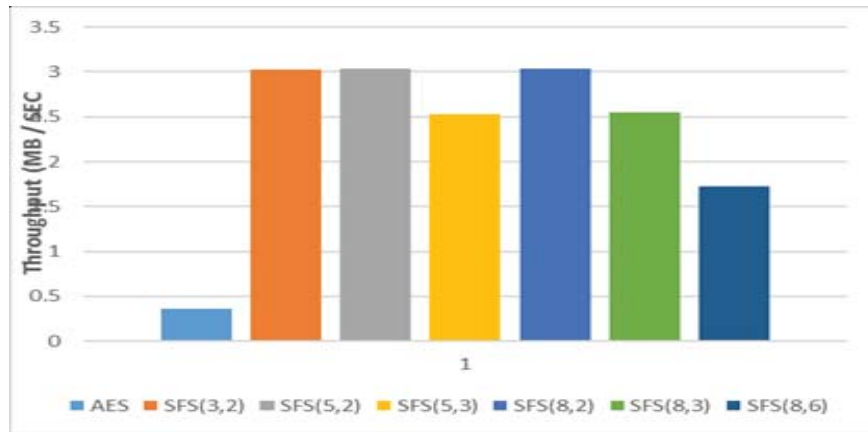
Figure 4.20: Throughput of the Sequential Execution Time of Reconstruct the Secret and Decryption using AES of most Popular File Formats.
