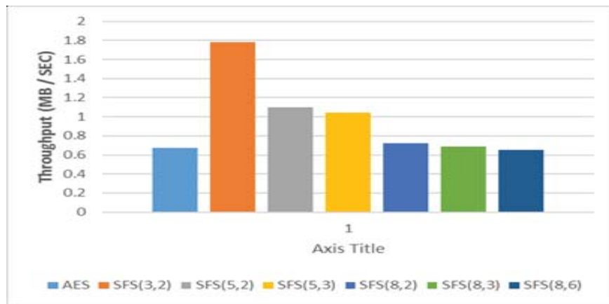
Figure A.12: Throughput of the Parallel Execution Time of Creating the Shares and Encryption using AES of Document File Type of Different Sizes.
