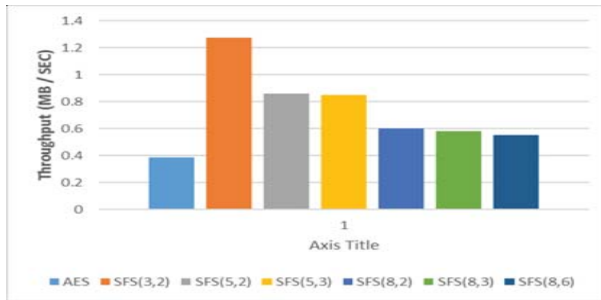
Figure A.22: Throughput of the Sequential Execution Time of Creating the Shares and Encryption using AES of Text File Type of Different Sizes.
