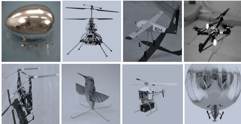
Figure 1.2 Aerodynamic Configurations (Top-Left to Bottom-Right): Blimp, Coaxial, Fixed-Wing, Quadrotor, Tandem rotors, Bird-like, Single rotor, Hybrid [6].
