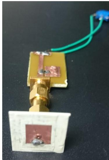
**Figure 5.20 Fabricated 2.43 GHz rectenna**
