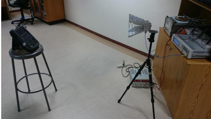
**Figure 5.18 Measurements Setup with 1 meter difference between the transmitter and the receiver**
