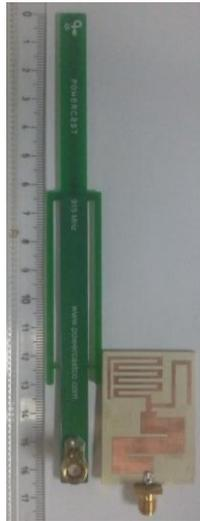
**Figure 4.29 Size comparison between the proposed MLA and the Powercast dipole antenna**
