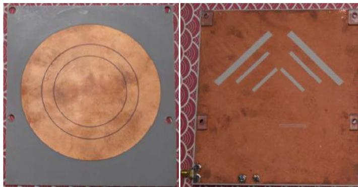
**Figure 3.30** the triple band circularly polarized antenna [50]
