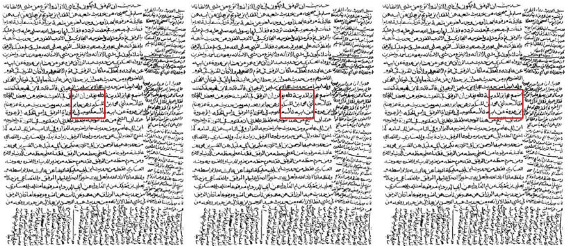
Figure 4.10: Sliding window text analysis, the window moves horizontally from left to right
