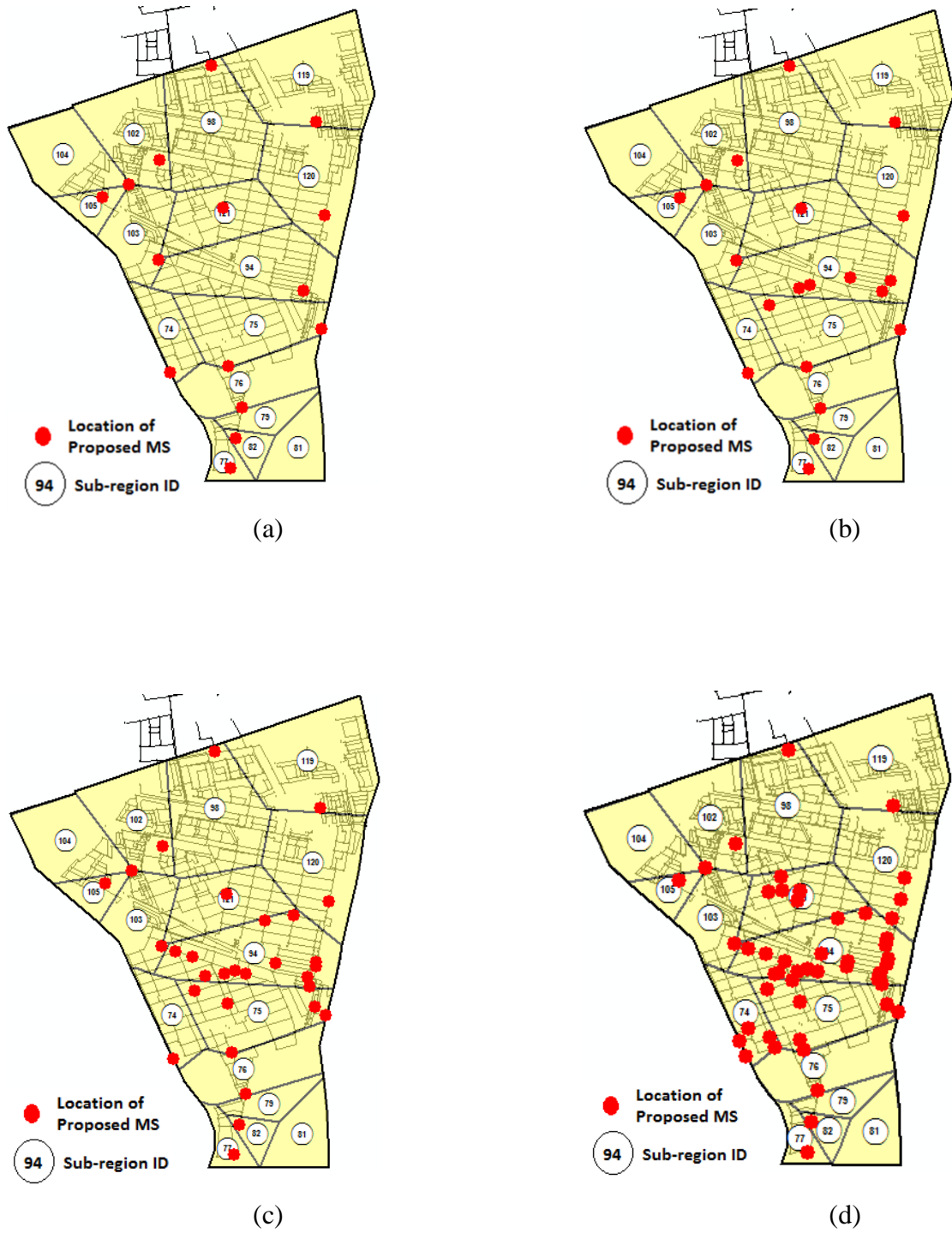
Figure 5.77 Optimal monitoring locations for 2nd 6 hours demand pattern and 60% CT based on vulnerability objective function for:
