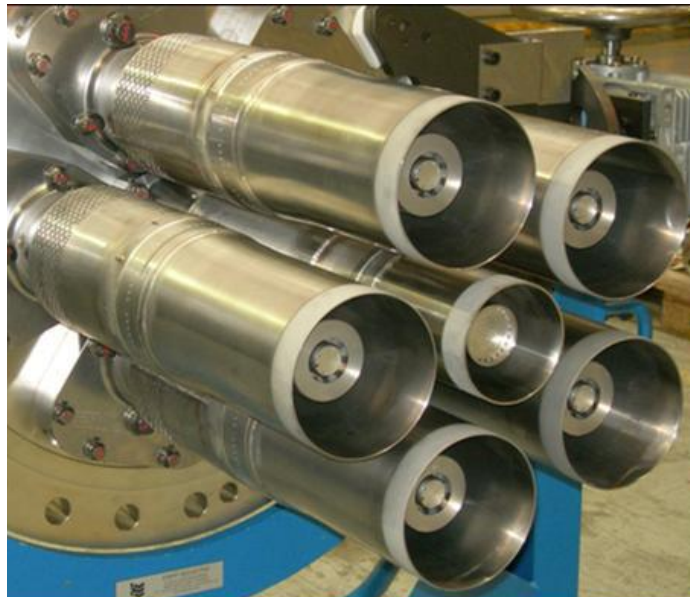
Figure 7 DLN-2.6 Combustor fuel nozzles
