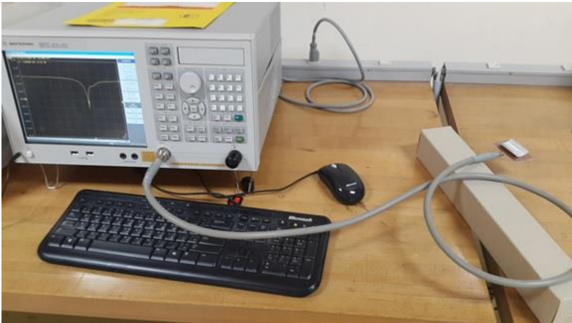
Figure 5-6: S_{11} Measurement of the Patch Antenna Using Vector Network Analyzer
