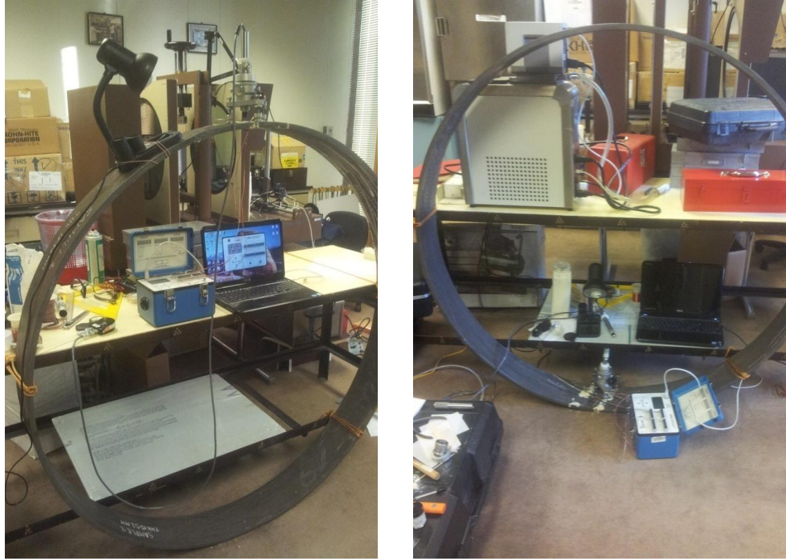
Fig. 6.8: Weld ring sample for residual stress measurement
