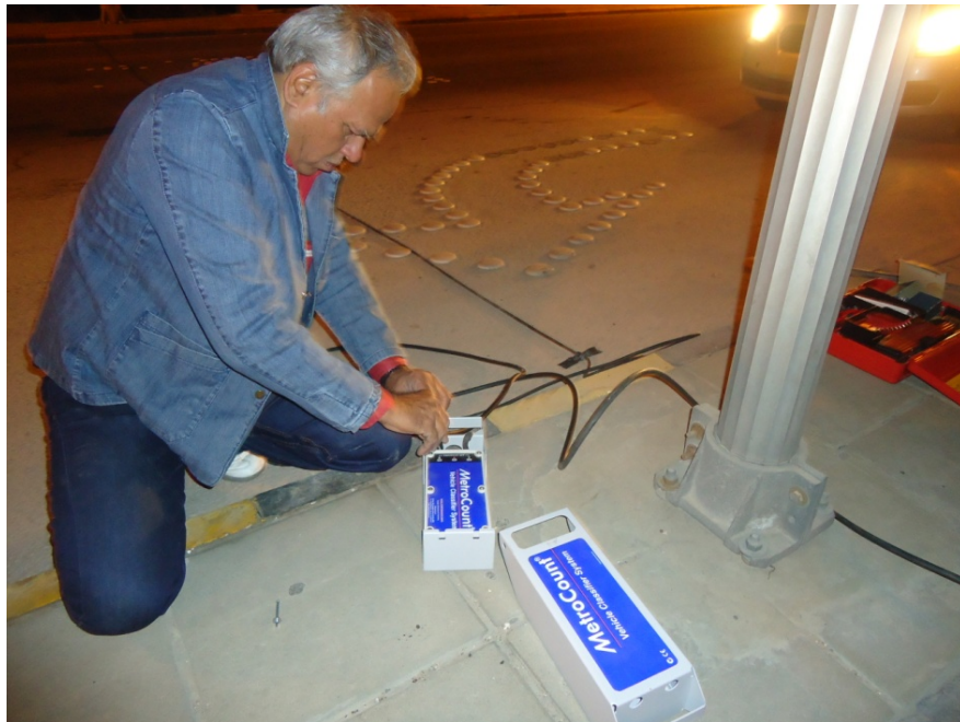
Figure 4-9 Setting up Automatic vehicle counter with the pneumatic tubes attached
