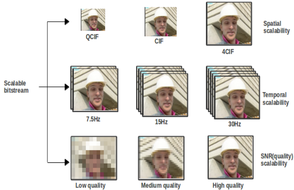
Figure 2.4: Types of scalability in video coding.
