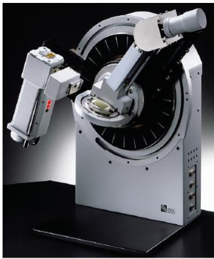
Figure 3.7: (a) D8 Bruker AXS X-ray diffractometer [www.bruker-axs.com], (b) basic geometry of Bragg-Brentano configuration and (c) GIXRD method. Note that the incident beam angle ( \omega ) is fixed during GIXRD analysis and the detector scans 2\theta degrees only.
