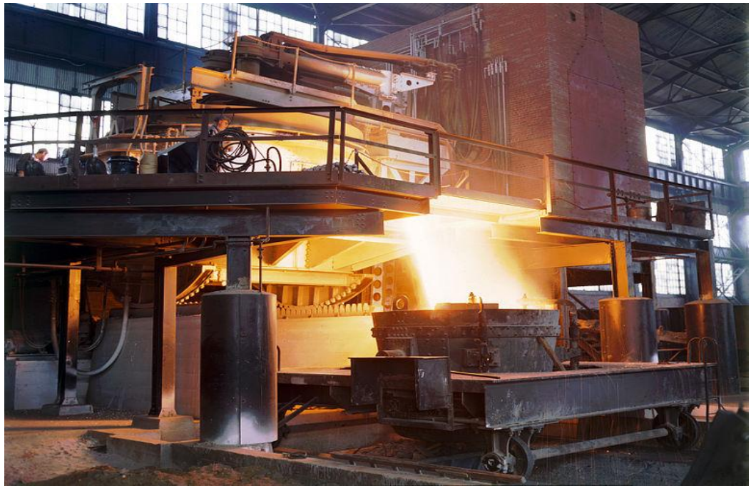
Figure 1.3: An electric arc furnace and the machines used in the steel making process.
